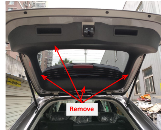
5. Remove the tailgate trim panels.
