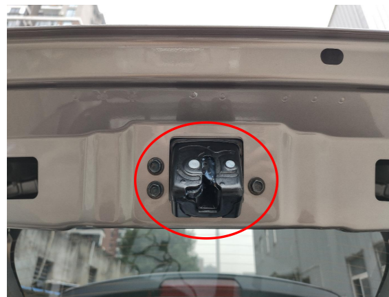
12. Remove the original latch and install our power latch.
