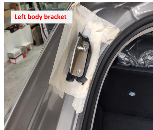
7. Replace the bracket on the left side of the trunk.
