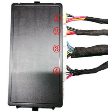
25. Insert the strut wiring harnesses ① ②, lock signal harness ③, and power harness ④ into the ECU in sequence, and then mount the ECU onto its bracket.
