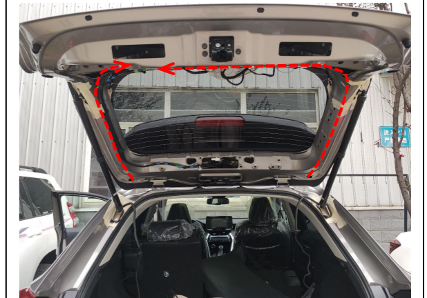
11. Route the strut wiring harnesses as indicated.
