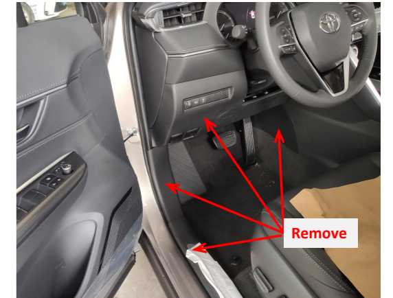
1. Remove the front left side door sill panels, switch panel and the trim panel on the right side of the driver's seat.
