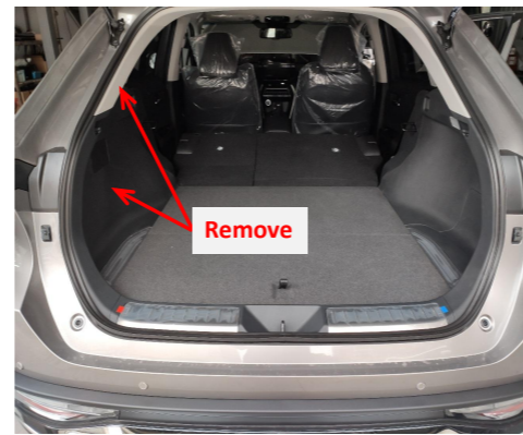
4. Take out the trunk floor mat and foam storage box. Remove the trim panels on the left side of the trunk to allow wiring harnesses to pass through.
