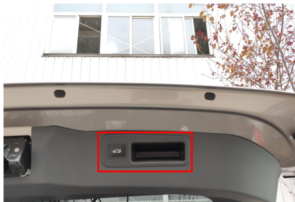
27. Reinstall all trim panel and install the added tailgate switch (replace the original handle).
