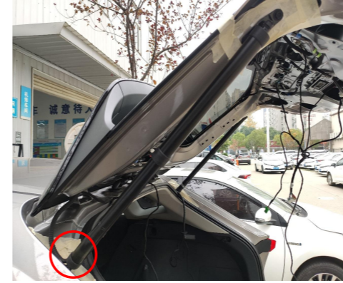
9. Install the electric struts, L on the left and R on the right (the first letter of the strut code), making sure the ends with wiring harnesses are on the car body.
