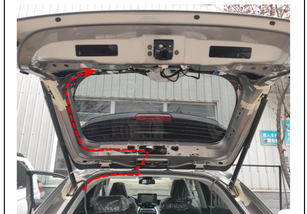
16. Thread the power harness to the tailgate.
