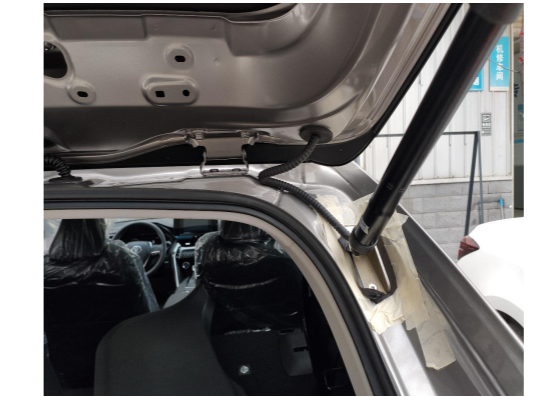
10. Thread the strut wiring harness through the hole into the tailgate and leave a certain length of rubber tube outside to prevent it from being bent during the movement of tailgate.
