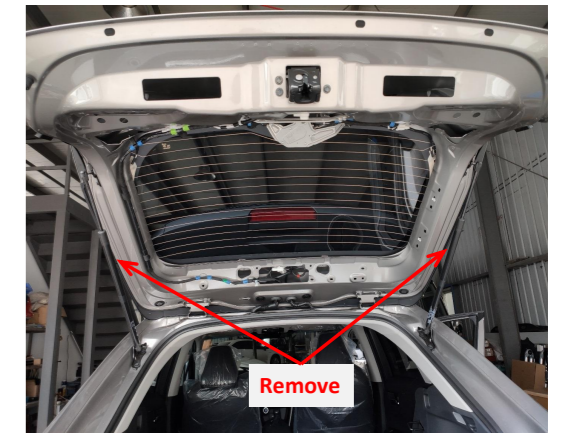
6. Remove the original gas struts.
