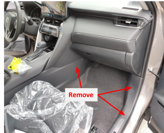
3. Remove the front right side door sill panels and the trim panel on the left side of the passenger seat.
