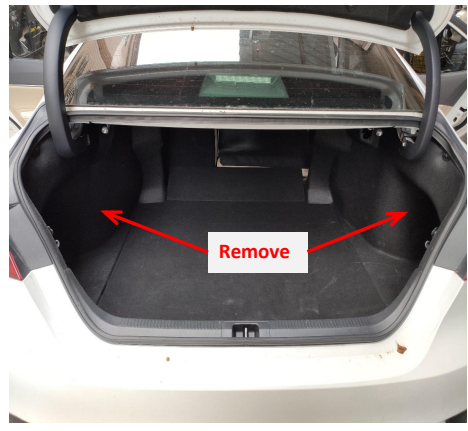
4. Take out the trunk floor mat and remove the trim panels on both sides of the trunk.
