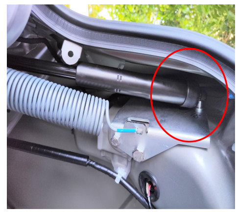
17. Install the electric struts, L on the left and R on the right (the first letter of the strut code), making sure the ends with wiring harnesses are on the car body.
