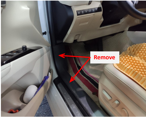
1. Remove the front left door sill panels.
