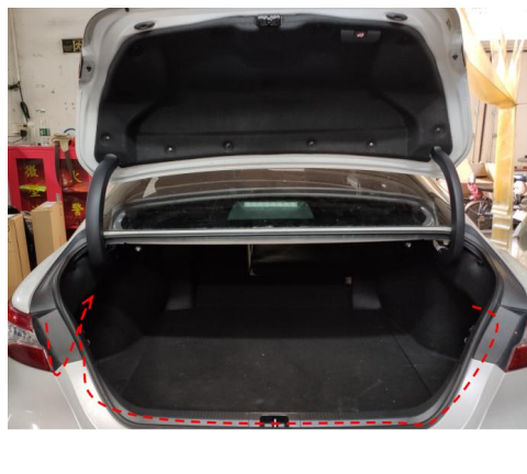
20. Route the right strut wiring harness along with orignal wires.
