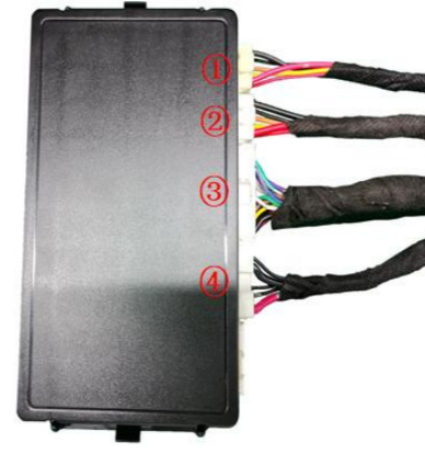
19. Insert the strut wiring harnesses ①②, lock signal harness ③, and power harness ④ into the ECU in sequence.
