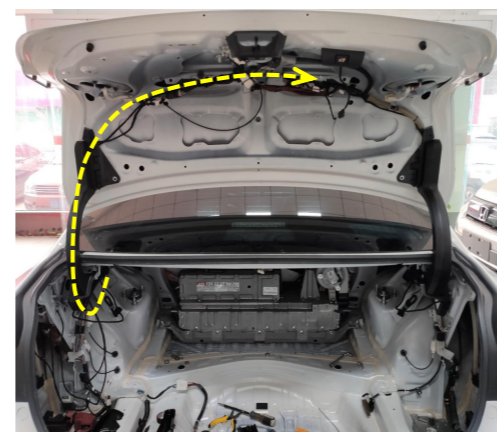
14. Route the power harness from the left hinge to the tailgate (routing only, no power connection).
