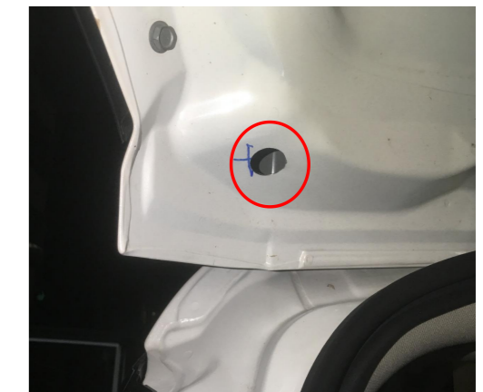
11. Drill a hole at the indicated position with a φ21mm drill to allow the strut wiring harnesses to pass through.
