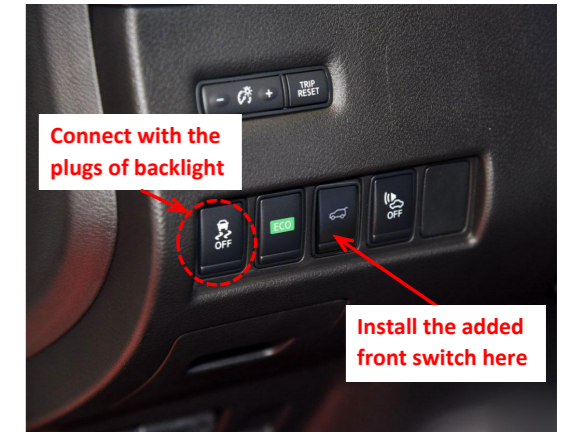
21. Remove the blank button, install the added front switch and connect with the plugs of backlight.
