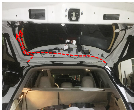
12. Thread the strut wiring harnesses to the tailgate.
