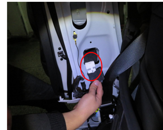
20. Connect the power harness to the indicated B-pillar signal plugs.
