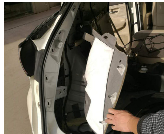
3. Remove the trim panel on the left side of the trunk to allow wiring harnesses to pass through.
