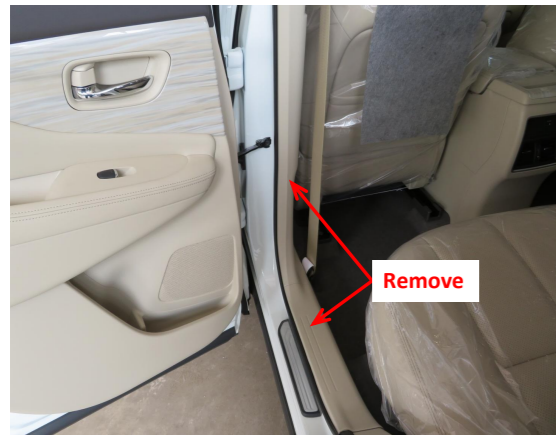
2. Remove the rear left side door sill trim panel and B-pillar trim panel.
