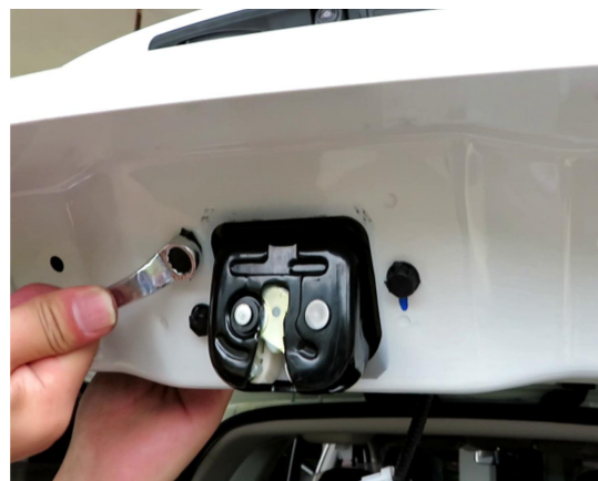
13. Remove the original latch and install our power latch.
