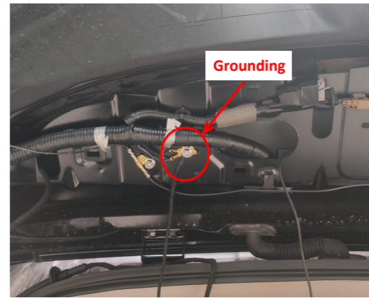
19. Ground at the top of the tailgate.
