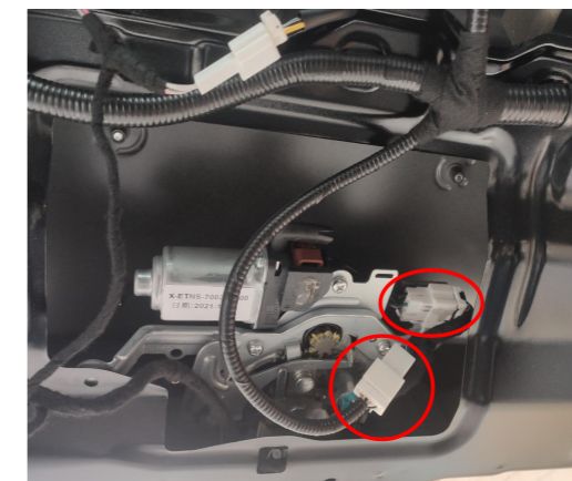
15. Connect the plugs of the lock signal harness to the plugs of the power latch.
