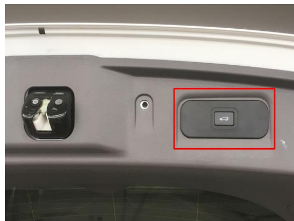
27. Reinstall all trim panels and install the added tailgate switch.
