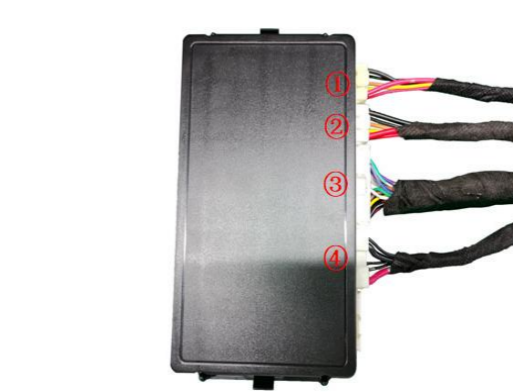
25. Insert the strut wiring harnesses ①②, lock signal harness ③, and power harness ④ into the ECU in sequence and then mount the ECU onto its bracket.
