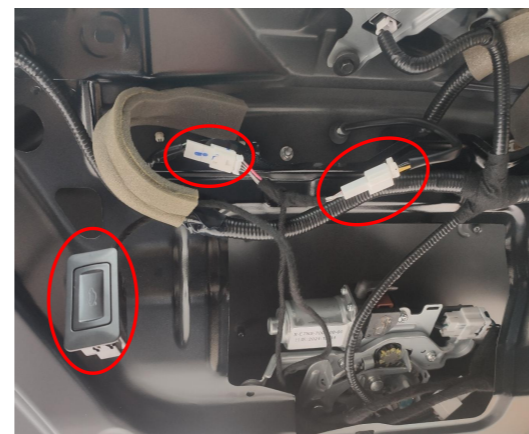
14. Connect the plugs of the lock signal harness to the plugs of the original tailgate switch and the added switch.
