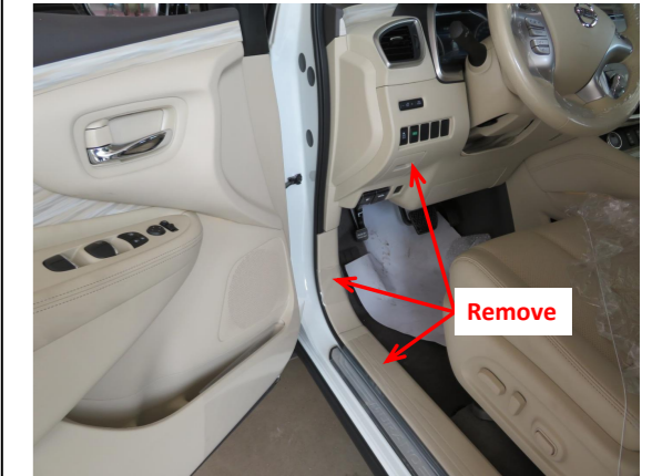
1. Remove the front left side door sill panel, switch panel and the exterior trim panel of the fuse box.
