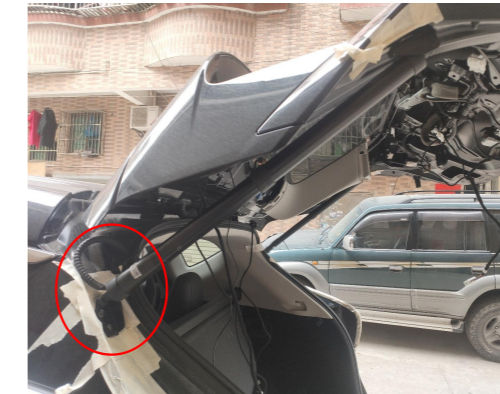
10. Install the electric struts, L on the left and R on the right (the first letter of the strut code), making sure the ends with wiring harnesses are on the vehicle body.
