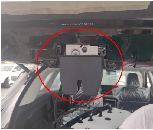
13. Remove the original latch.
