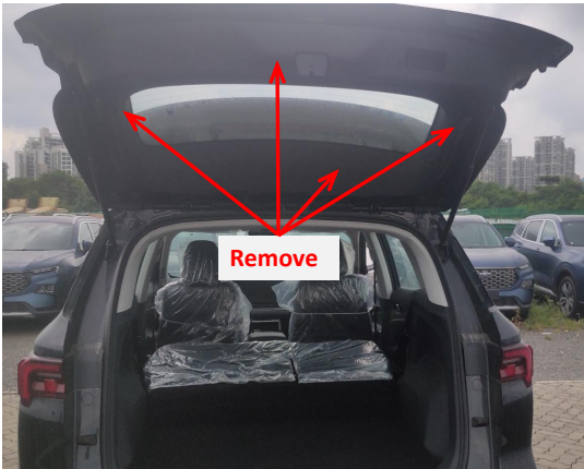
3. Remove the tailgate trim panel.
