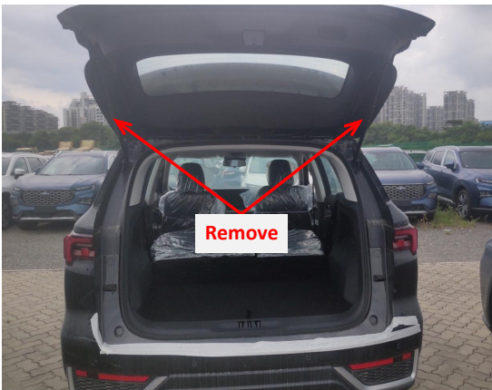
5. Remove the original gas struts.
