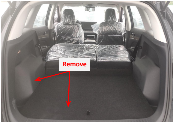
4. Take out the trunk floor mat and the trim panel on the left side to allow the wiring harnesses to pass through.
