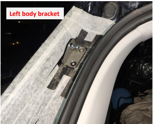
6. Replace the left body bracket.
