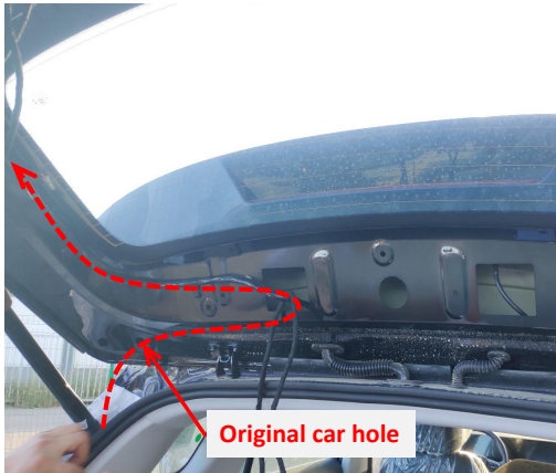
9. Thread the strut wiring harnesses through the holes on both sides.
