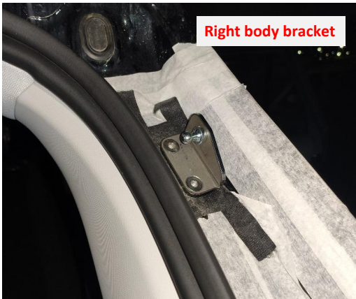
7. Replace the right body bracket.
