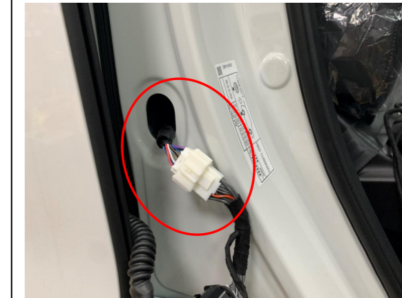
21. Connect the power harness to the indicated B-pillar signal plugs
