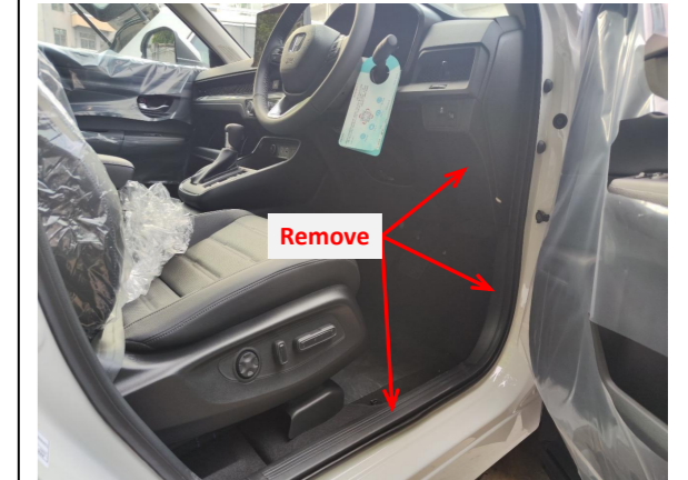
1. Remove the front right side trim panels and door sill panel.
