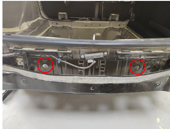
8. Thread the wiring harnesses through the holes of the bumpers.
