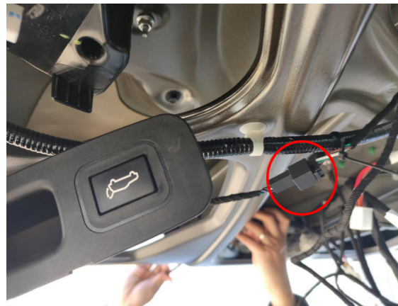
17. Connect the plug of the lock signal harness to the added tailgate switch.
