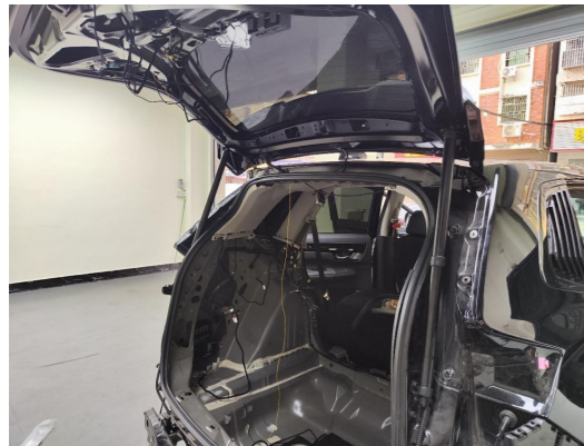
7. Install the electric struts, L on the left R on the right (the first letter of the strut code), making sure the ends with wiring harnesses are on the car body.
