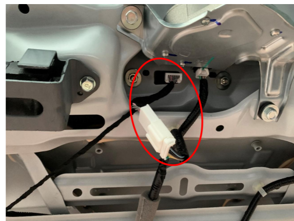
18. Connect the plugs of the lock signal harness to the plugs of the original tailgate switch.
