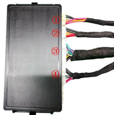
28. Insert the strut wiring harnesses ①②, lock signal harness ③, and power harness ④ into the ECU in sequence.
