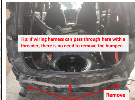
5. Remove the bumpers (if wiring harness can pass through here with a threader, there is no need to remove the bumper).
