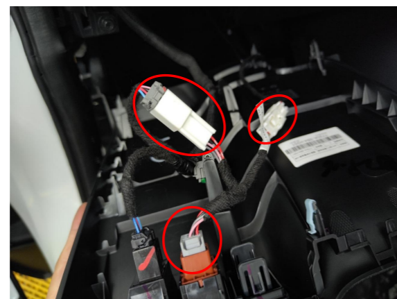
23. Connect the plugs of the power harness to the plugs of the added front switch and the switch beside it for backlight.
