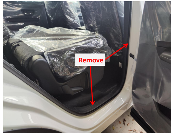
2. Remove the rear right door sill panel and the B-pillar trim panel
