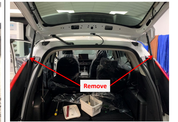
6. Remove the gas struts.
