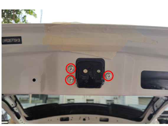
13. Remove the original latch and install the power latch.
