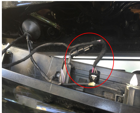
11. Connect the plugs of the lock signal harness to the plugs of tailgate handle switch.
