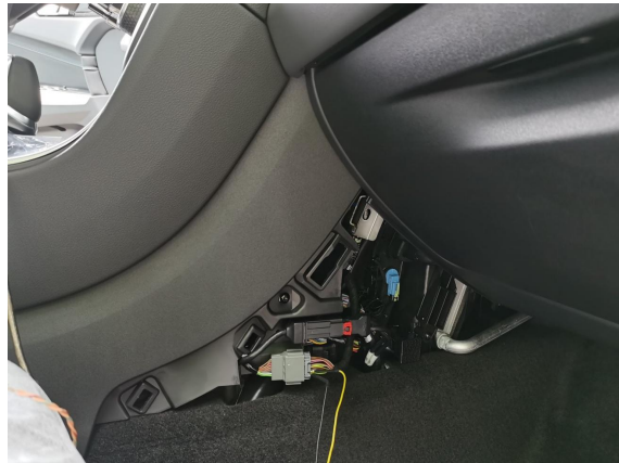
1. Remove the trim panel on the left side of the passenger seat.
