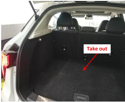
4. Take out the trunk floor mat and the foam storage box.
