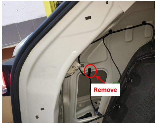
27. Remove the indicated cable clip on the left side of the trunk for installing the ECU.
