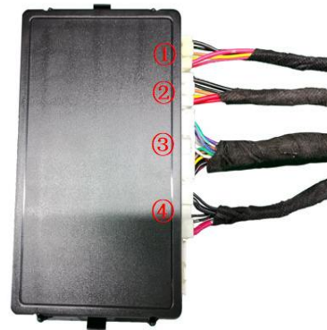
28. Insert the left and right strut wiring harnesses ①②, lock signal harness ③, and power harness ④ into the ECU in sequence. Then fit the ECU into its bracket.
