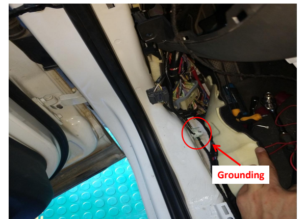
21. Ground at the indicated position on the left side of the driver's seat.
