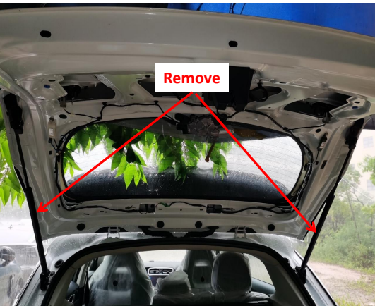
15. Remove the original gas struts.
