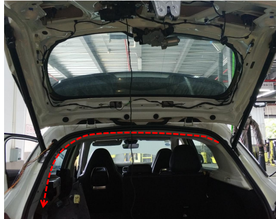
18. Thread the strut wiring harness into the car body and route the them to the left side of the trunk.
