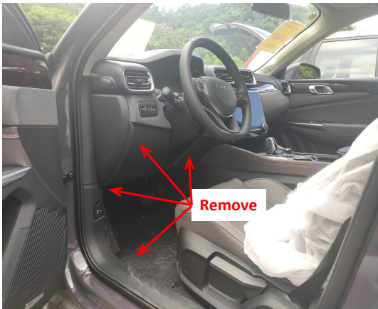
2. . Remove the indicated driver's side trim panels.
