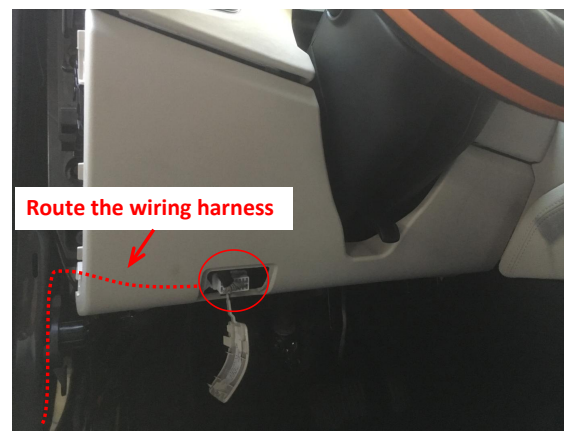
23-2. For gas version: connect to the OBD plug at the driver's area.
