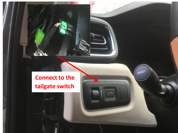
22. Connect the plugs of the power harness to the front tailgate switch.
