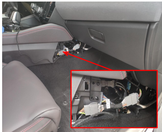
23-1. For hybrid version: connect plugs of the power harness to the CAN plugs on the left side of the passenger
