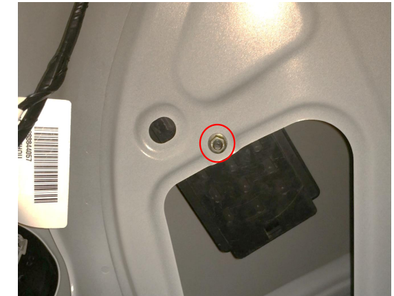
29. Secure the ECU with a nut.
