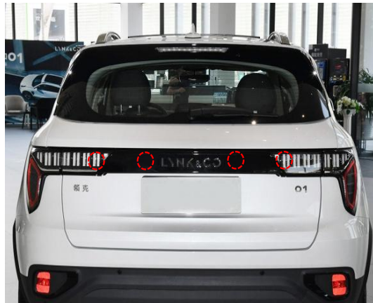
7. Remove the tailgate handle trim panel (there are screws in the circles).
