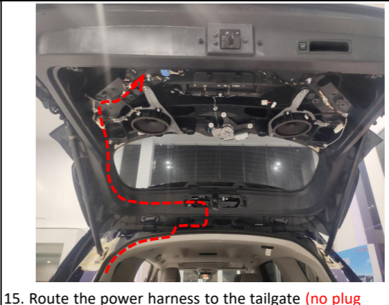
15. Route the power harness to the tailgate (no plug connection before inserting terminals into wiring harness connector).
