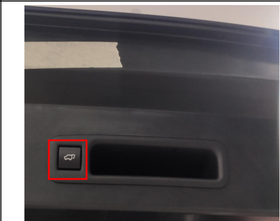
26. Reinstall all the trim panels and install the added tailgate switch.
