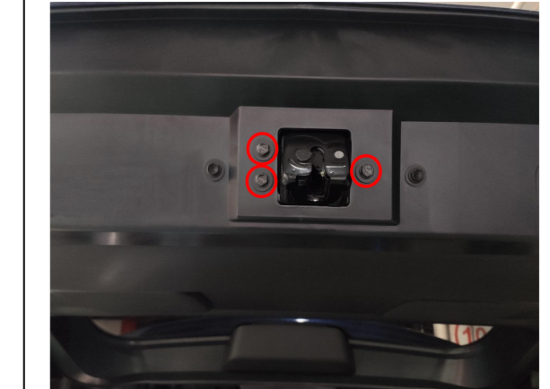
11. Replace the original latch with our power latch.
