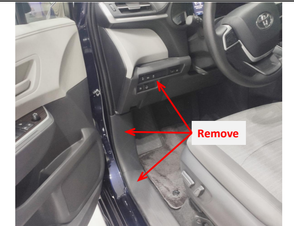
1. Remove the front left door sill panels, switch panel and storage box.
