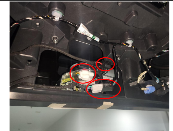
13. Connect the lock signal harness to the plugs of the power latch.
