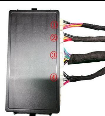
24. Insert the strut wiring harnesses ① ②, lock signal harness ③, and power harness ④ into the ECU in sequence, and then mount the ECU on its bracket.
