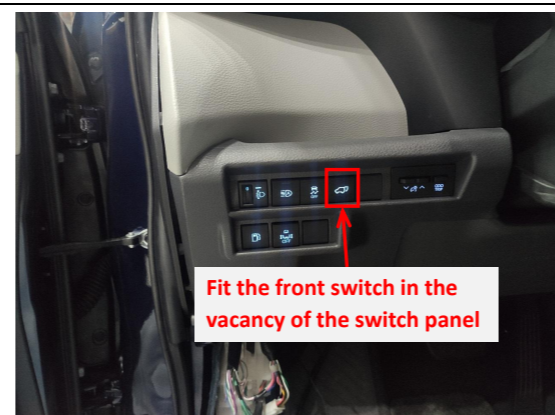
19. Remove the blank button from the switch panel to install the added front switch and then connect proper plugs for backlight behind the switch panel.
