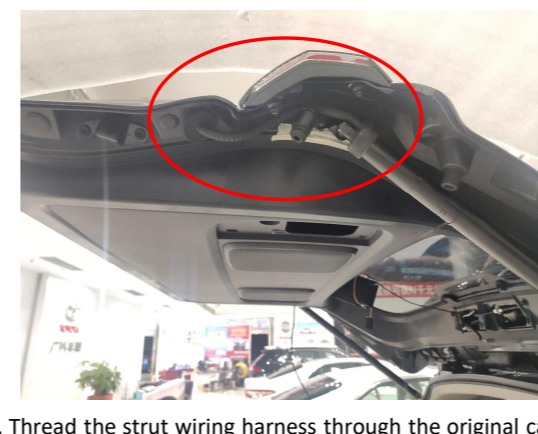
9. Thread the strut wiring harness through the original car hole into the tailgate, plug the hole tightly and then place the rubber tube between the bump stop and the tailgate.
