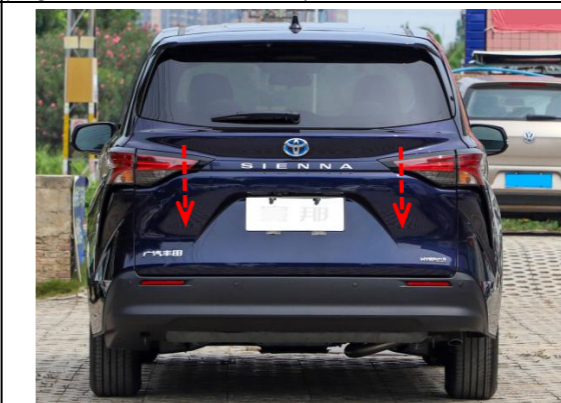
25. Press the tailgate buttons to open and close the tailgate once, the system completes initialization, and then test each function of the electric tailgate.
