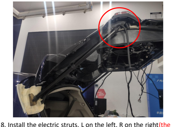
8. Install the electric struts, L on the left, R on the right (the first letter of the strut code), making sure the ends with wiring harnesses are on the tailgate.
