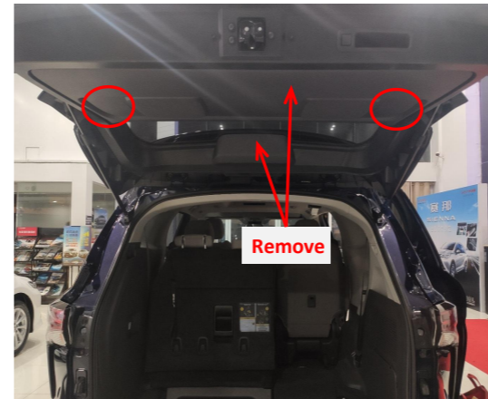
4. Remove the tailgate trim panels (there are two small trim panels with screws at the circled position).
