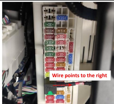
22. Plug the fuse tap into the fuse box and pay attention to the direction.
