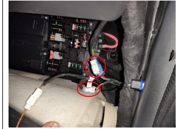
21. Connect the power harness to the signal plugs on the right side of the passenger seat.
