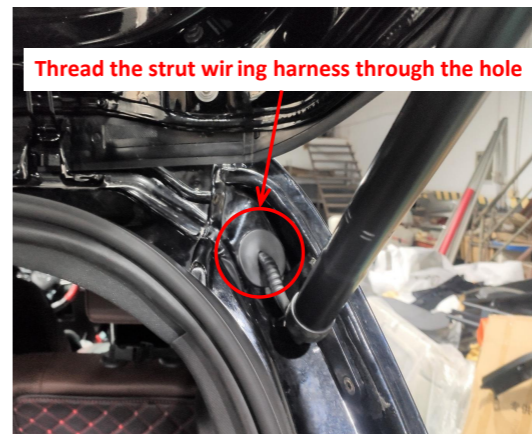
10. Thread the strut wiring harness through the indicated hole into the tailgate.
