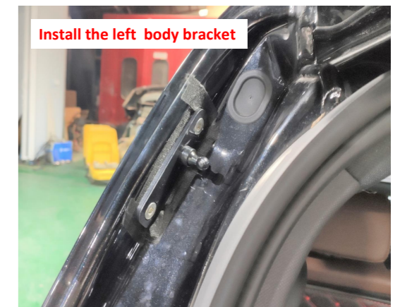
6. Install the left body bracket.
