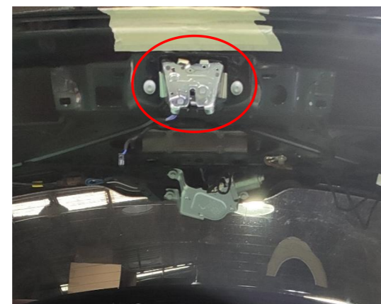
13. Remove the original latch.
