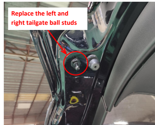
8. Replace the ball studs on the left and right sides of the tailgate.
