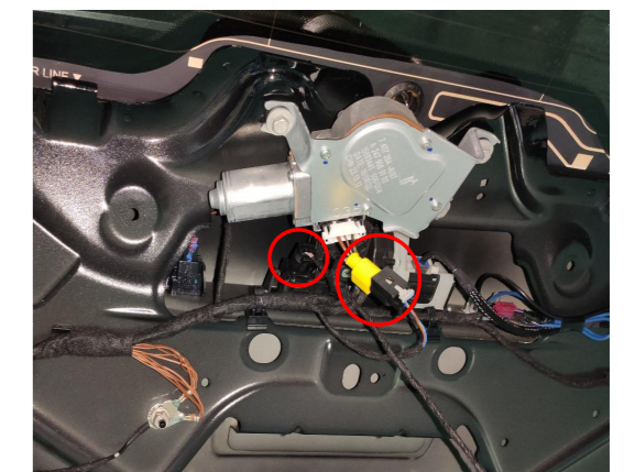
16. Connect the lock signal harness to the plugs of the original tailgate switch and the added tailgate switch.
