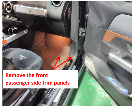
2. Remove the trim panels on the right side of the passenger seat.
