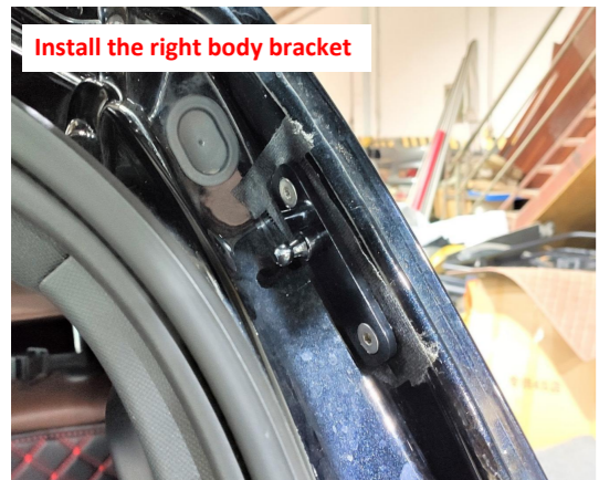
7. Install the right body bracket.
