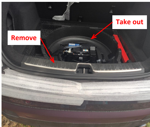
5. Remove the indicated trim panel and foam storage box.
