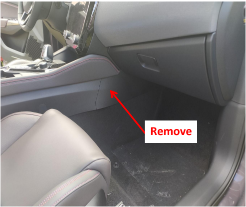
1. Remove the trim panel on the left side of the passenger seat.
