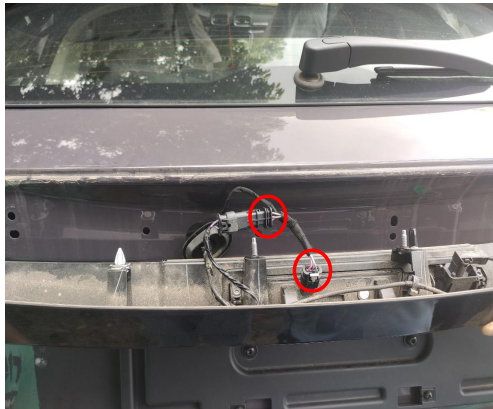
12. Connect the plugs of the lock signal harness to the plugs of tailgate handle switch.
