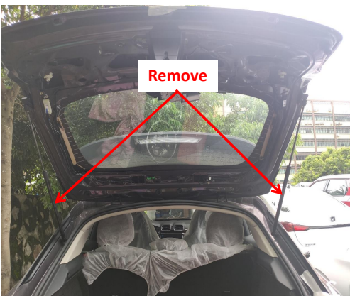
18. Remove the original gas struts.
