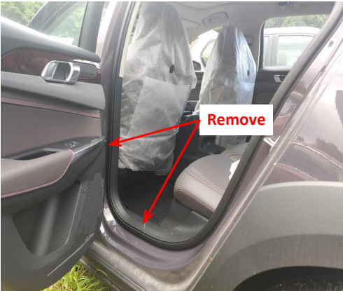
3. Remove the rear left door sill panel and B-pillar trim panel.
