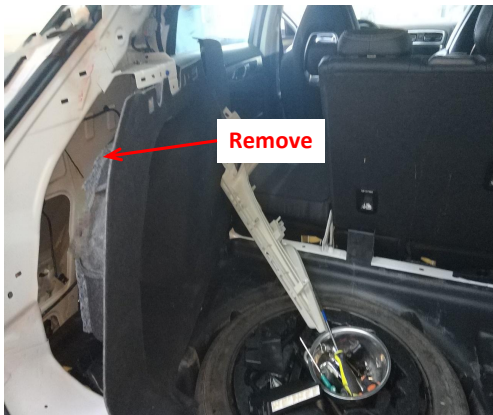
6. Remove the trim panel on the left side of the trunk.
