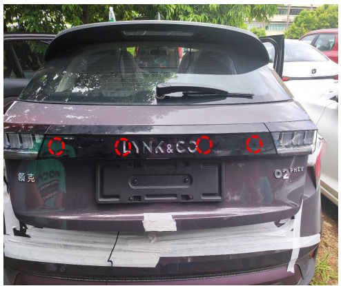
8. Remove the tailgate handle trim panel (there are screws in the circles).
