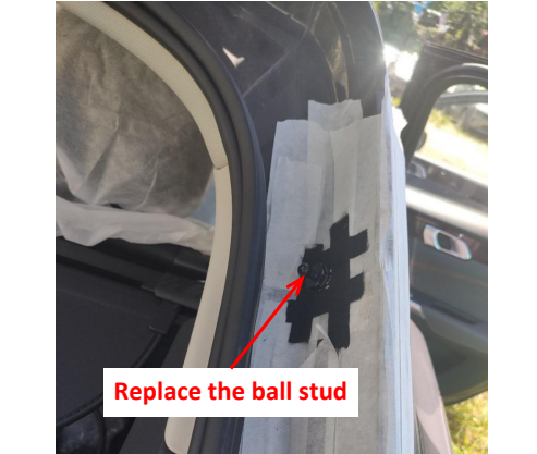
19. Replace the ball studs on both sides of the car body.
