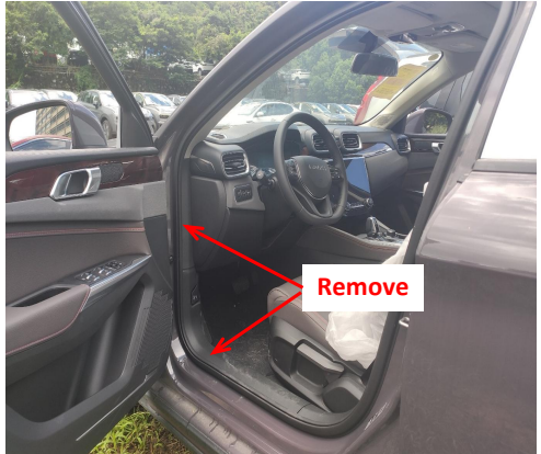
2. Remove the indicated driver's side trim panels.
