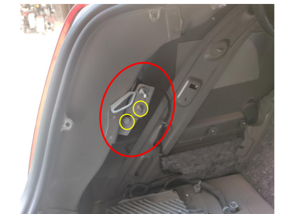
13. Install the bracket at the left side of the trunk (use two bolts to secure the bracket).
