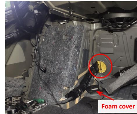
9. Remove the foam cover from the left side of the trunk and thread the emergency wires of the lock signal harness through the hole to the rear seat.
