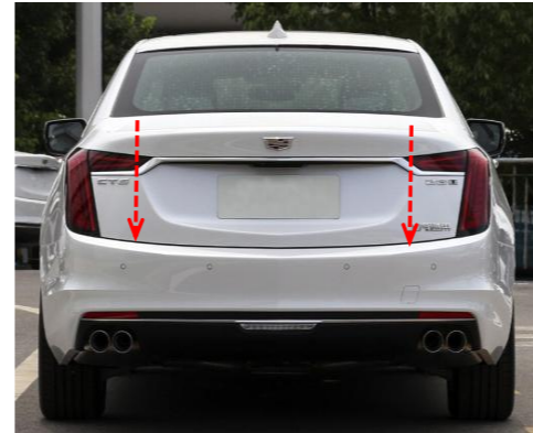
24. Press the added tailgate switch button to open and close the tailgate once for initializing the system, and then test the functions of the electric tailgate.
