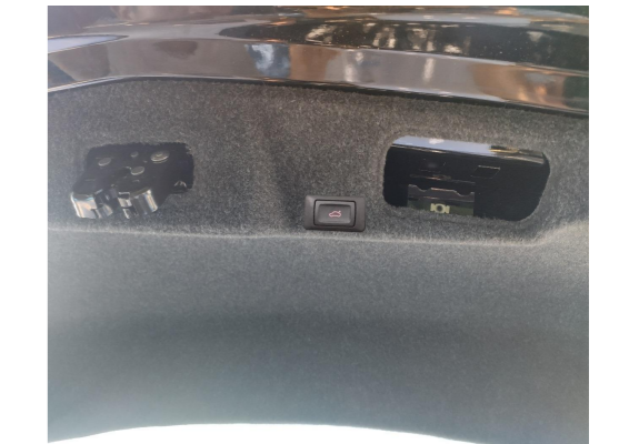
26. Reinstall all the trim panels and install the added tailgate switch.
