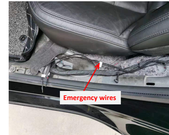
10. Hide the emergency wires under the rear left side door sill panel.
