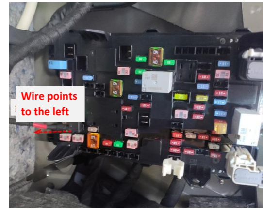
20. Move the original fuse from the slot to fuse tap, and then plug the fuse tap into the fuse box; pay attention to the direction.
