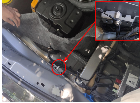
18. Ground with the power harness at the right side of the trunk.
