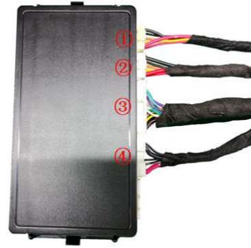
23. Insert the strut wiring harnesses ① ②, lock signal harness ③, and power harness ④ into the ECU in sequence and then mount the ECU onto its bracket.
