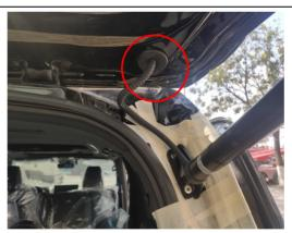
9. Thread the strut wiring harness into the tailgate through the circled hole, and then plug the hole with the hole plug. Both sides follow the same method.
