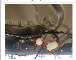
12. Connect the lock signal harness to the plugs of the power latch.
