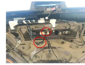
11. Connect the lock signal harness with the plugs of the original tailgate switch. (Two pairs of plugs are reserved, choose the appropriate one according to the original plugs)
