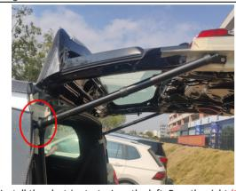
8. Install the electric struts, L on the left, R on the right (the first letter of the strut code), making sure the ends with wiring harnesses are on the vehicle body.
