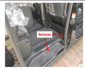
2. Remove the rear right door footstep to allow wiring harnesses to pass through.
