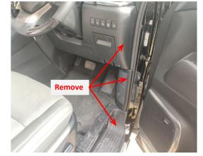
1. Remove the indicated driver's side trim panels and footstep.
