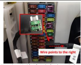
21. Move the original fuse from the fuse box to the fuse tap and then plug the fuse tap into the fuse box. Pay attention to the direction.
