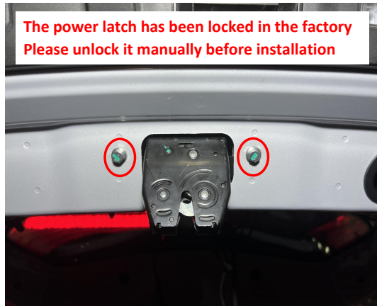
14. Install the power latch with the provided screws.
