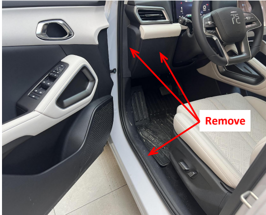
1. Remove the front left door sill panel and the trim panels of the fuse box.
