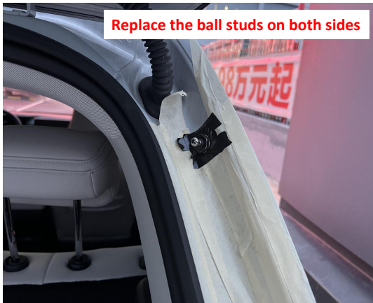
6. Replace the ball studs on both sides.
