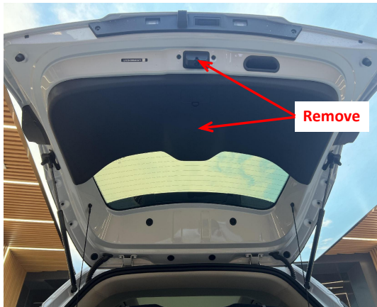
4. Remove the trim panels on the tailgate.
