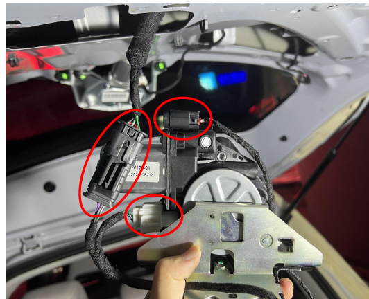
13. Connect the plugs of the lock signal harness to the power latch.
