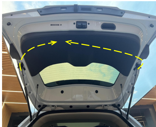
10. Thread the left and right strut wiring harnesses to the indicated position.
