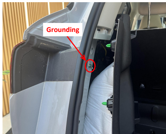
16. Ground at the indicated position on the left side of the trunk.
