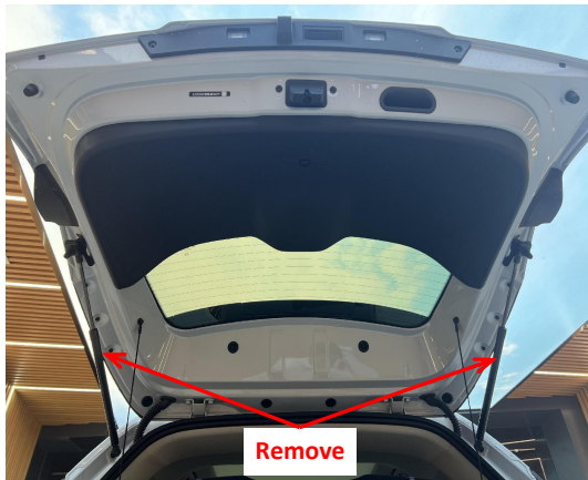
5. Remove the original gas struts.
