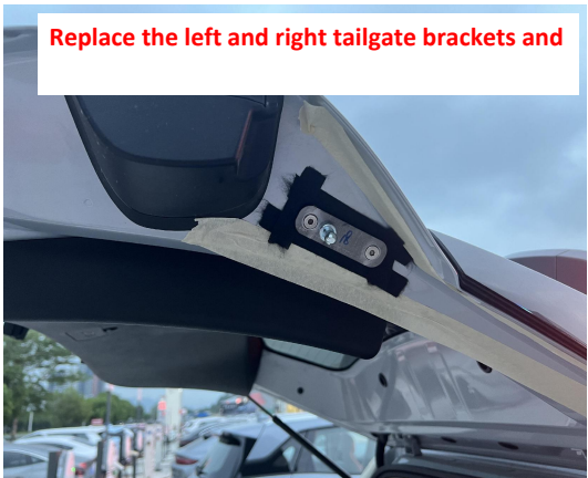
7. Replace the left and right tailgate brackets.
