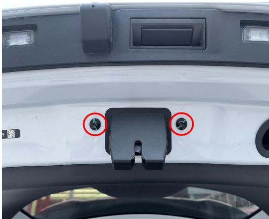
11. Remove the plastic casing of the latch and remove the latch.
