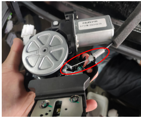
17. Install the original emergency cable onto the power latch (there are two fasteners. Choose the outer fastener)
