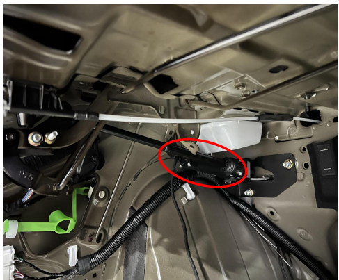
13. Install the left strut (L&R are marked as the first letter of the strut code).
