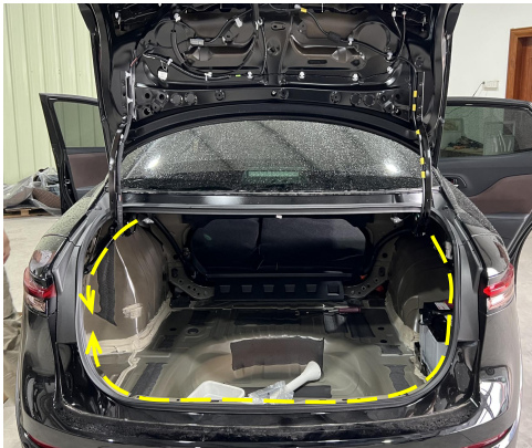
15. Route the strut wiring harnesses to the left side of the trunk along with the original wires.
