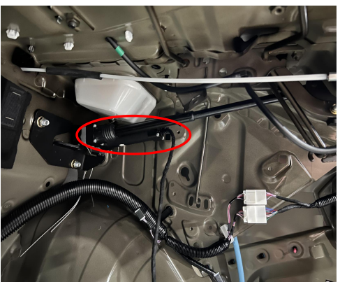
14. Install the left strut (L&R are marked as the first letter of the strut code).
