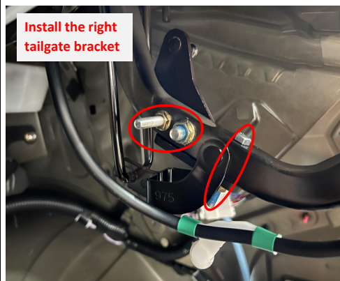
12. Install the right tailgate bracket on the right hinge.
