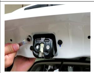
13. Remove the original latch and install our power latch.
