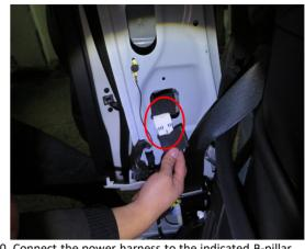
20. Connect the power harness to the indicated B-pillar signal plugs.
