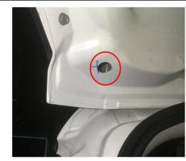
to allow the strut wiring harnesses to pass through.
