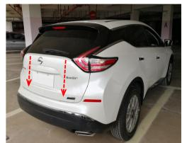
26. Press the added tailgate switch button to close the tailgate once for initializing the system and then test each function of the electric tailgate.
