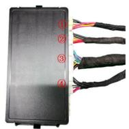
harness (3), and power harness (4) into the ECU in seguence and then mount the ECU onto its bracket.
