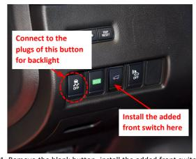
21. Remove the blank button, install the added front switch button and connect the plugs of backlight.
