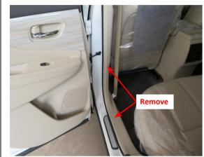
2. Remove the rear left side door sill trim panel and B-pillar
