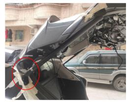
10. Install the electric struts, L on the left and R on the right (the first letter of the strut code), making sure the ends with 11. Drill a hole at the indicated position with a φ21mm drill wiring harnesses are on the vehicle body.
