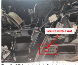
24. Place the ECU bracket at the indicated position and secure it with a nut.
