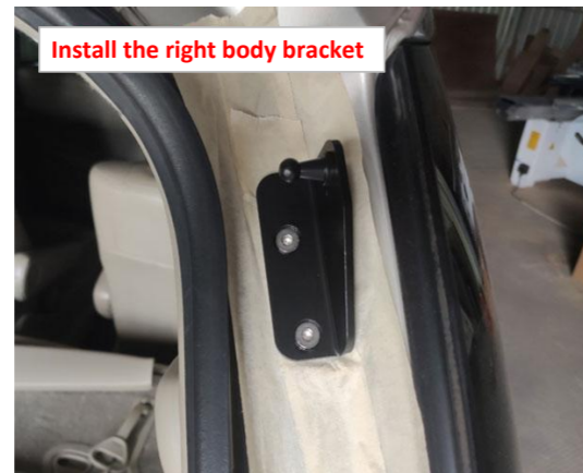
8. Install the right body bracket.
