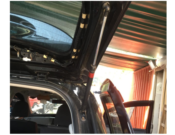
6. Remove the gas struts (remove the screws from the bracket).
