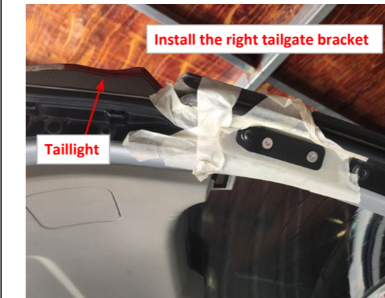
10. Install the right tailgate bracket.
