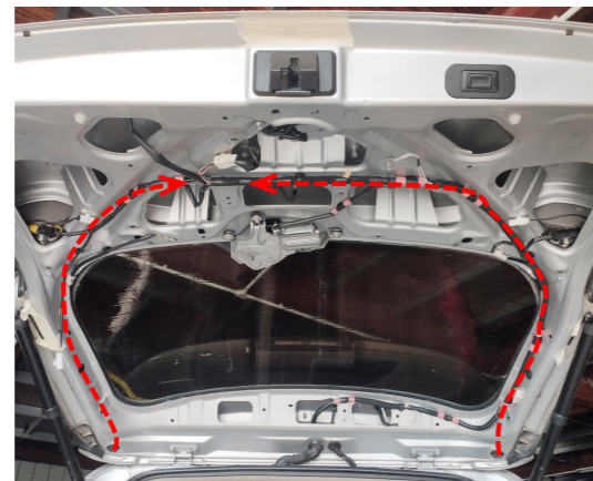
13. Route the strut wiring harnesses.
