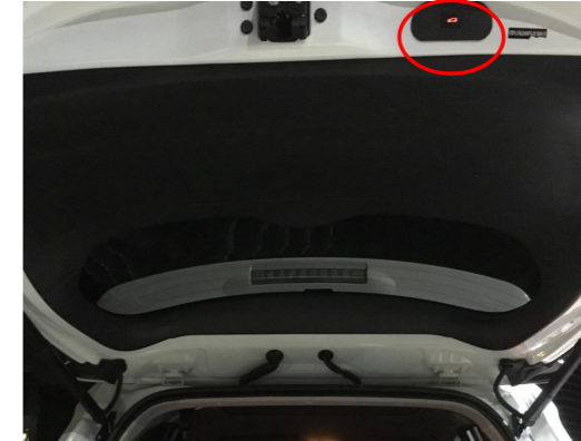
25. Reinstall all the trim panels and install the added tailgate switch.
