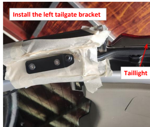
9. Install the left tailgate bracket.
