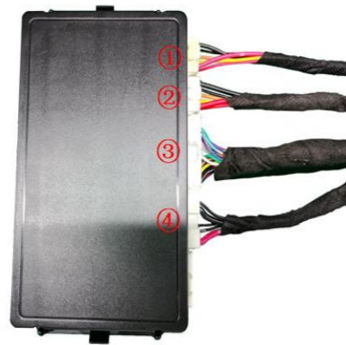
23. Insert the strut wire harnesses ① ②, lock signal harness ③, and power harness ④ into the ECU in sequence, and then mount the ECU on its bracket.
