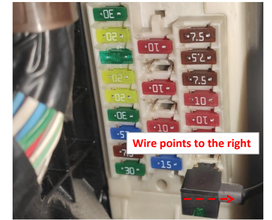
21. Plug the fuse tap into the fuse box and pay attention to the direction.
