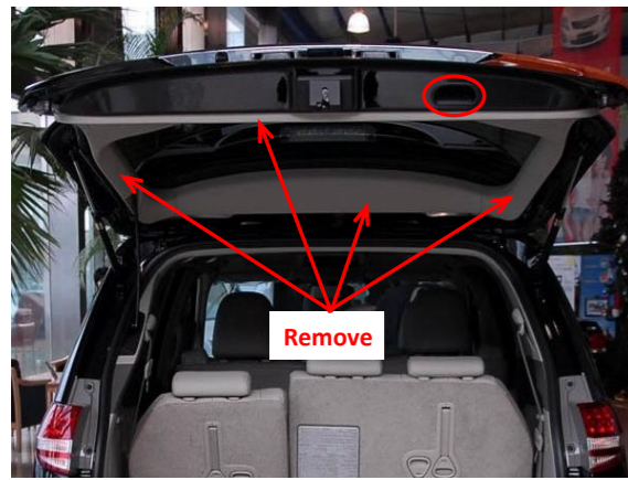
2. Remove the the tailgate trim panels.
