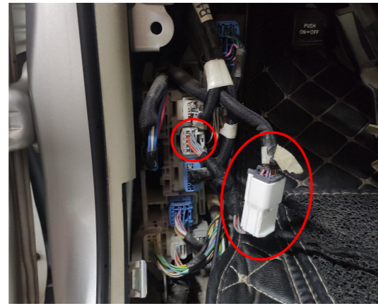
18. Connect the power harness to the signal plug and its socket.
