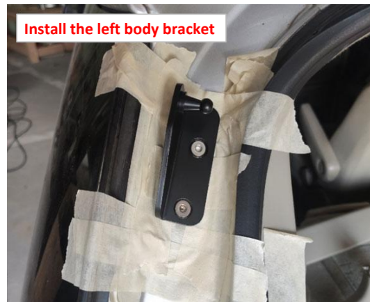
7. Install the left body bracket
