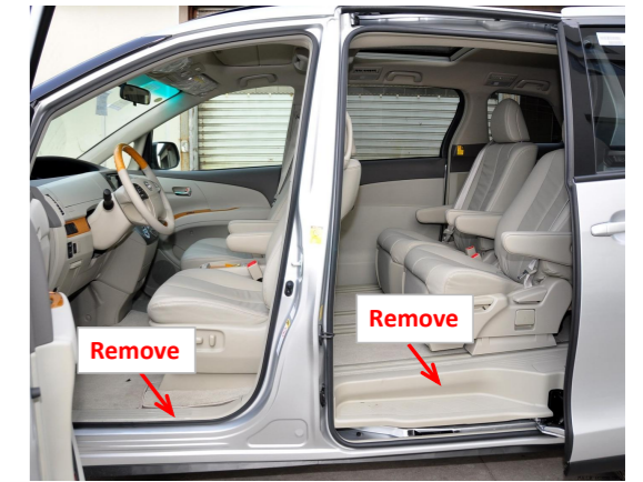
1. Remove the left side door sill panels to allow wiring harnesses to pass through.
