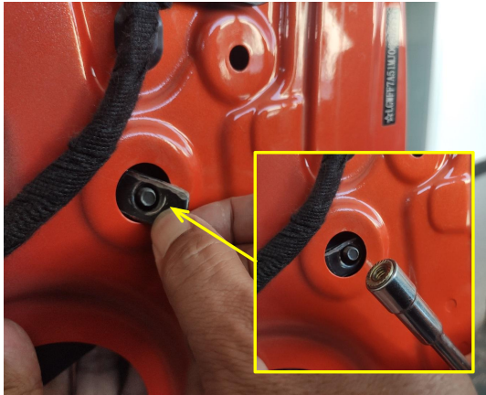
23. Use a nut to secure the shim.
