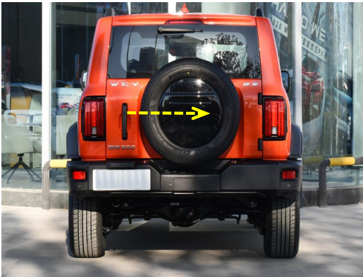
26. Press the added tailgate switch to open and close the tailgate once, the system completes initialization, and then test each function of the electric tailgate.
