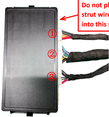
24. Insert the left and right strut wire harnesses①, lock signal harness②, and power harness③ into the ECU in sequence.
