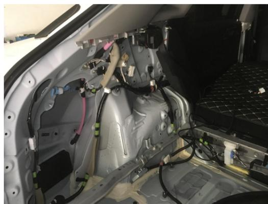
7. Remove the trim panel on the left side of the trunk to allow wiring harnesses to pass through.
