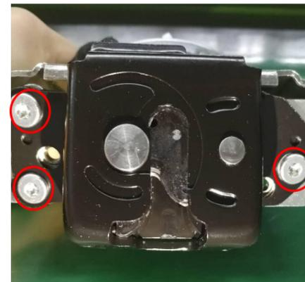
9. Remove the screws from the power latch.
