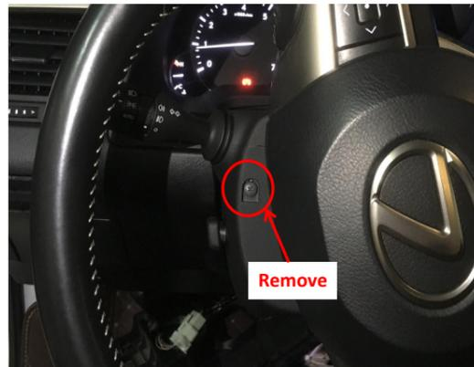
2. Remove the screws on the left and right sides of the steering wheel.
