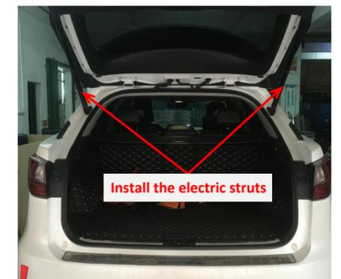
16. Install the electric struts, L on the left and R on the right (the first letter of the strut code).
