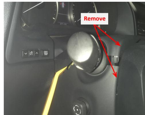
3. Remove the upper and lower trim panels of the steering column.
