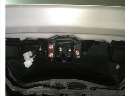
10. Remove the original lock and install the power latch.
