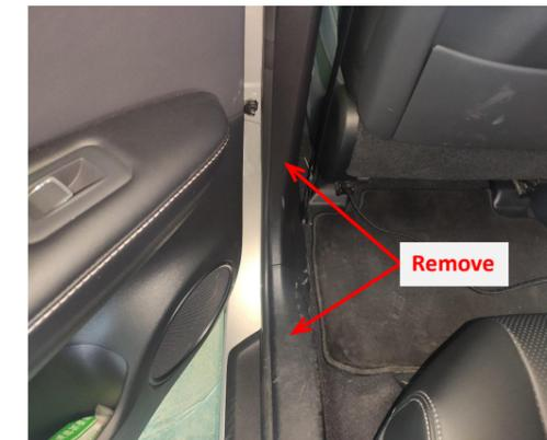
5. Remove the rear left side door sill panel and B-pillar trim panel.
