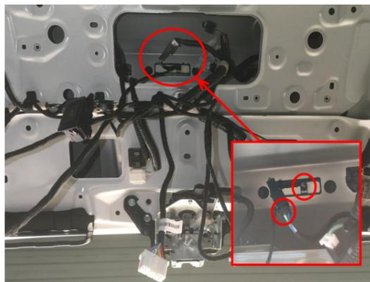
12. Connect the lock signal harness to the original tailgate switch and its plug.
