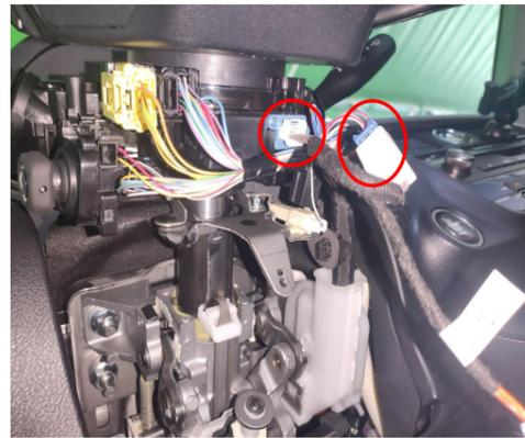
23. Connect to the blue signal plug and its socket at the steering column.
