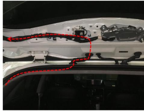
19. Thread the power harness to the tailgate (do not connect plugs before inserting terminals into wiring harness connector).
