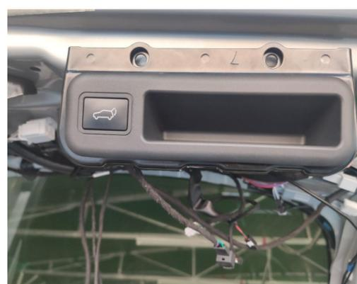
13. Install the added switch at the tailgate handle
