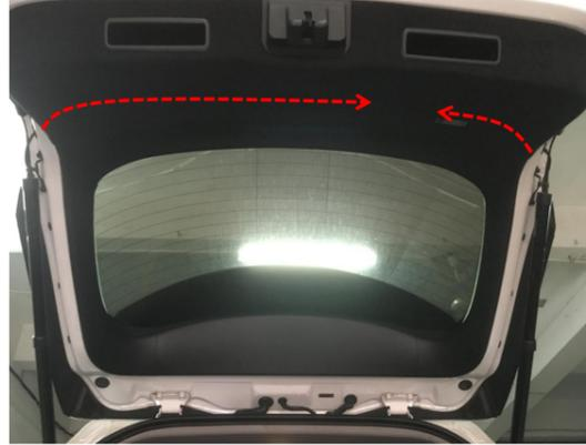
18. Route the strut wiring harnesses.
