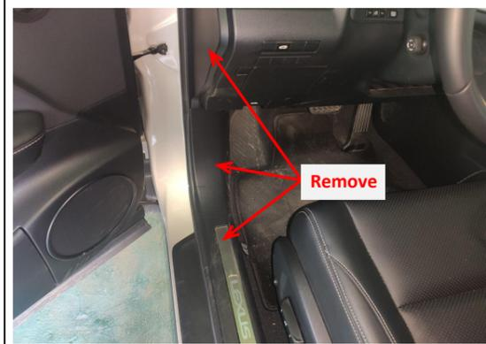
4. Remove the front left side trim panels and door sill panel.
