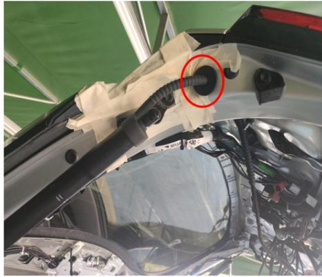
17. Pass the strut wiring harness through the original square hole and then plug the hole. Both sides are the same.
