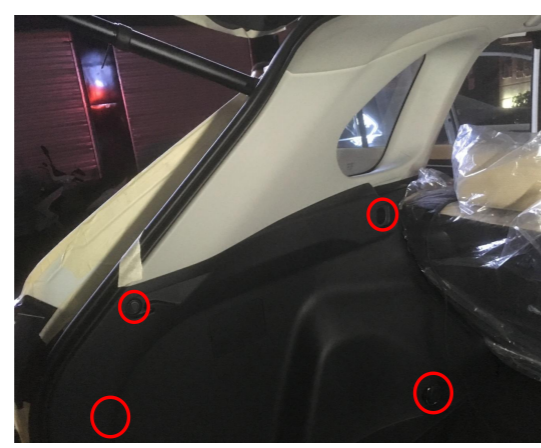
3. Remove the trim panel on the left side of the trunk (there are screws in the circles).
