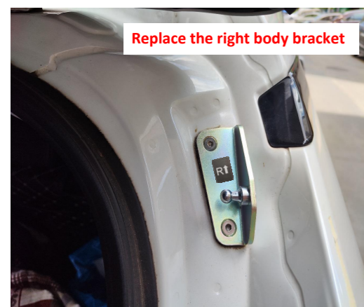
12. Replace the right body bracket.
