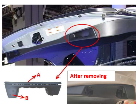
28. Remove the indicated tailgate handle (After removing part A, unscrew the screws, and then remove part B).
