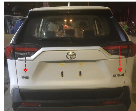
27. Initialize the system once, and then test each function of the electric tailgate.
