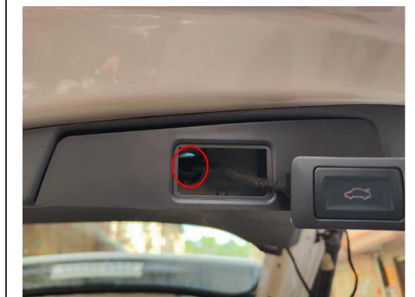
31. Install the tailgate switch trim panel (install the screw) and the tailgate switch.
