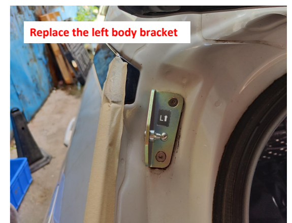
11. Replace the left body bracket.
