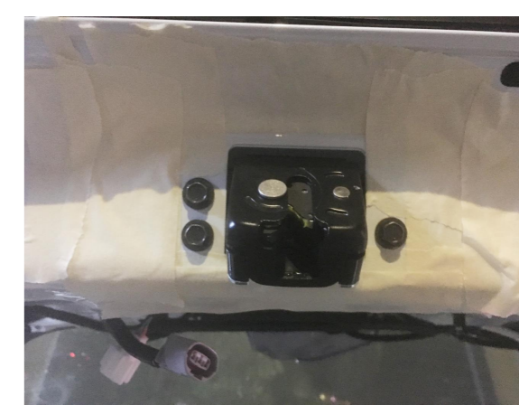
6. Remove the original latch and install our power latch.
