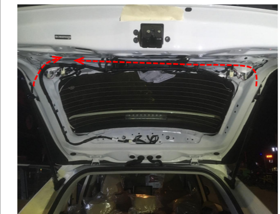
14. Thread the strut wiring harnesses through the holes into the tailgate and route them as shown above.
