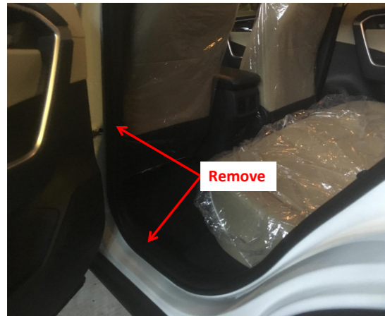
2. Remove the rear left B-pillar trim panel and door sill panel.
