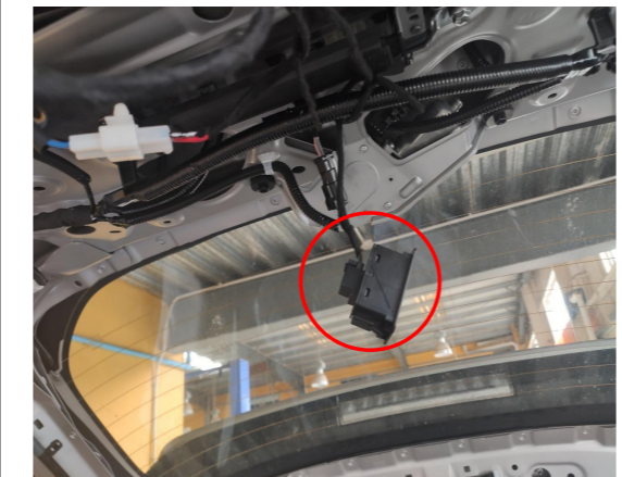
9. Install the added tailgate switch (the switch shown above is for test, and the actual switch may be different).
