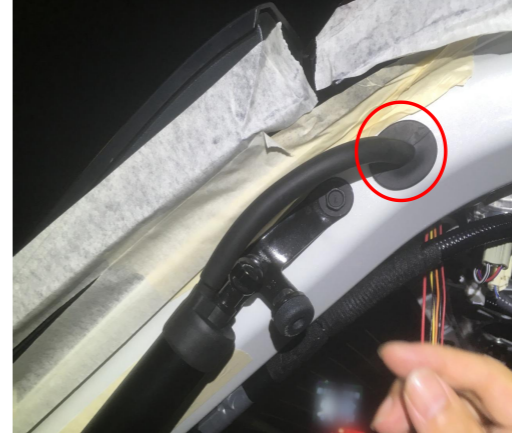
15. Plug the left and right holes with rubber plugs.
