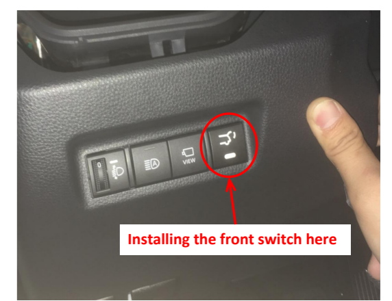
21. Install the added front switch at the reserved place of the switch panel.
