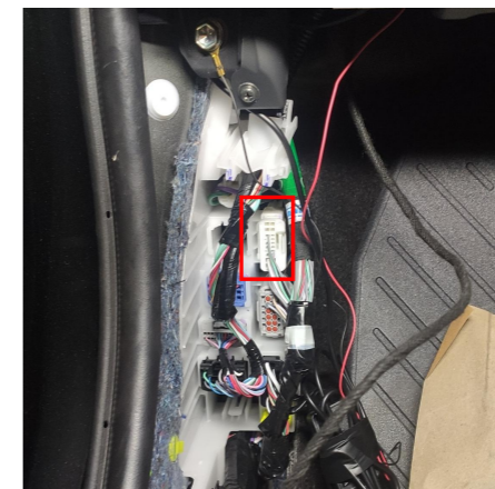
20. Connect the power harness to the signal plug and its socket at the front passenger's area
