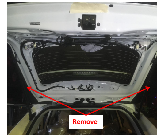
10. Remove the gas struts.
