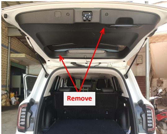
3. Remove the tailgate trim panels.
