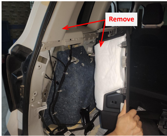
5. Remove the indicated trim panels on the left side of the trunk to allow wiring harnesses to pass through.
