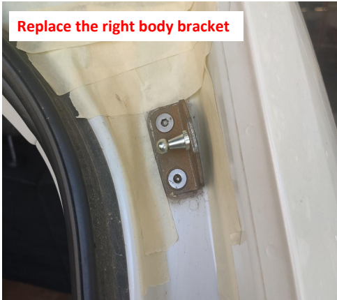
8. Replace the right body bracket.
