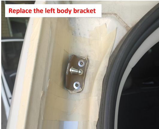
7. Replace the left body bracket.
