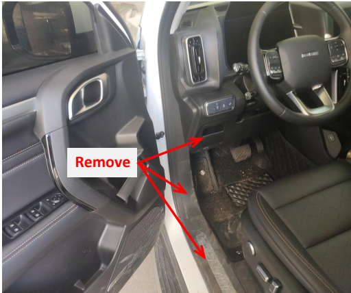
1. Remove the front left door sill panels and storage box.
