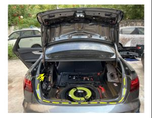
13. Route the strut wiring harnesses to the left side of trunk. 14. Remove the original latch.
