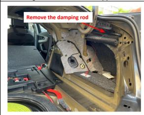
. Remove the damping rod.
