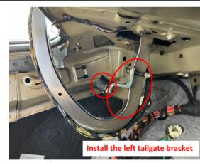
8. Install the left tailgate bracket and provided bump stop. For the right hinge, only replace the bump stop.
