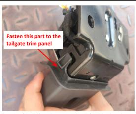
29. Fasten the latch casing securely to the tailgate trim panel
