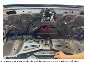
18. Connect the lock signal harness to the plugs of the original tailgate switch.
