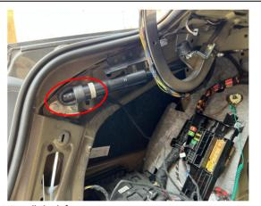
10. Install the left strut (L&R are marked as the first letter of the trut code). Pay attention to the location of rubber tube.
