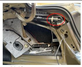
11. Install the left strut (L&R are marked as the first letter of the strut code). Pay attention to the location of rubber tube.
