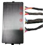
24. Insert the left and right strut wiring harnesses (1)(2), lock signal harness (3), and power harness (4) into the ECU
