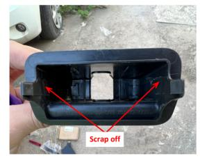
28. Scrap off the indicated ribs of the original latch casing.
