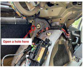
22. Drill a hole at the indicated location with a φ6mm drill
