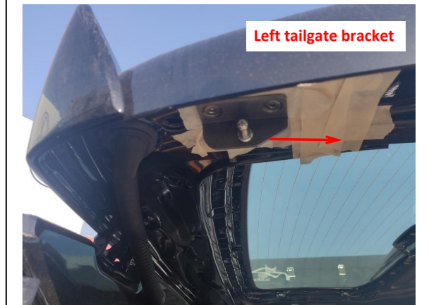
6. Replace the left tailgate bracket.
