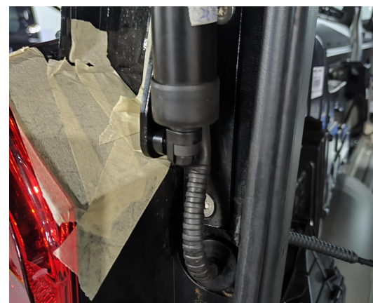
12. Thread the strut wiring harness into the car body and plug the hole securely.
