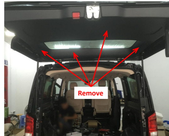
4. Remove the tailgate trim panels.
