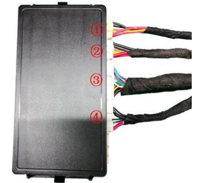
26. Insert the strut wiring harnesses ①②, lock signal harness ③, and power harness ④ into the ECU in sequence and then fit the ECU onto its bracket.
