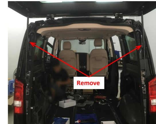
5. Remove the original gas struts.
