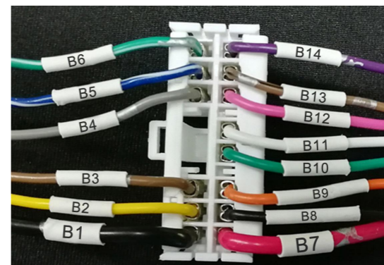
15. Insert the lock signal harness terminals into the wiring harness connector according to the diagram. Note: For models with fewer than 14 wires, just insert them according to the corresponding label or color.
