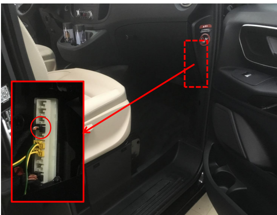
22. Plug in the signal plug at the right side of the passenger storage box.
