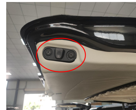
30. Replace the left and right bump stops.
