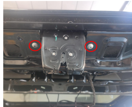
18. Secure the power latch.
