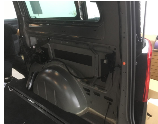
3. Remove the trim panel on the right side of the trunk to allow the strut wiring harnesses to pass through.
