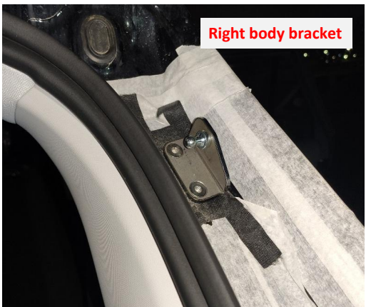
7. Replace the right body bracket.
