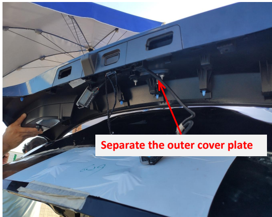
15. Separate the outer cover plate of the tailgate.
