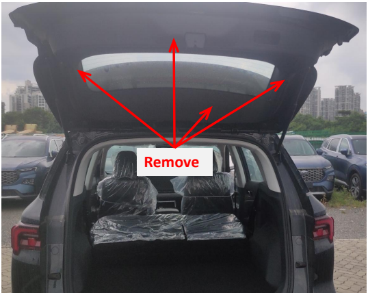
3. Remove the tailgate trim panel.
