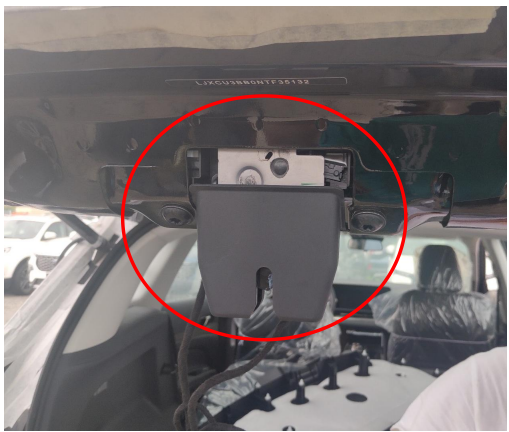
13. Remove the original latch.
