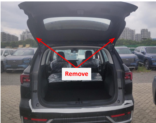
5. Remove the original gas struts.
