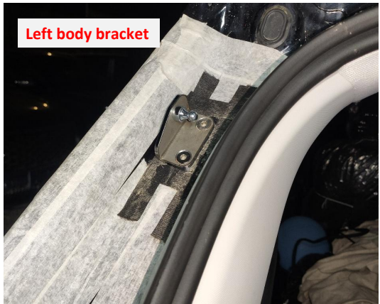
6. Replace the left body bracket.
