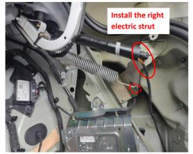
13. Install the right electric strut and hang the right spring back. (pay attention to hang the spring to the indicated hole)
