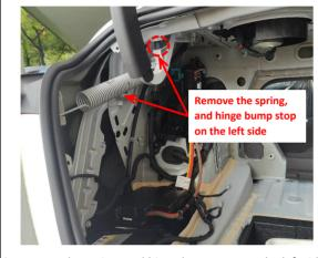
3. Remove the spring, and hinge bump stop on the left side.
