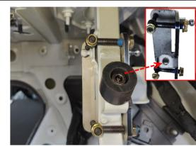
6. Secure the right bracket with the rubber mounting bolt, pass the eye-bolts through the bracket, and pass the hex socket bolts through the holes of the eye-bolts, then tighten the nuts.
