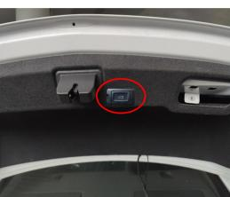
26. Install the added tailgate switch and reinstall all the trim
