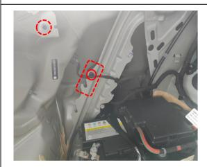
7. Locate the indicated holes on the left side of the trunk.
