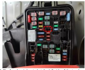
20. The fuse box is located at the left side of the trunk and the fuse slot for power supply is indicated above.
