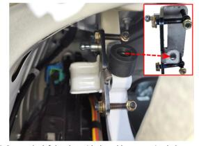
5. Secure the left bracket with the rubber mounting bolt, pass the eye-bolts through the bracket, and pass the hex socket bolts through the holes of the eye-bolts, then tighten the nuts.
