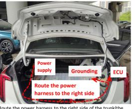
18. Route the power harness to the right side of the trunk(the routing method of the strut wiring harnesses are the same with the oower harness)
