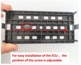
22. Pass the screw through the bracket and mount the ECU
