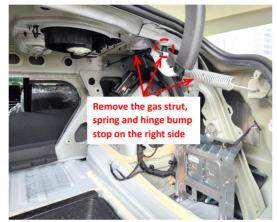
Remove the gas strut, spring and hinge bump stop on the
