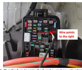
21. Plug the fuse tap into the fuse box and pay attention to the direction of wire.
