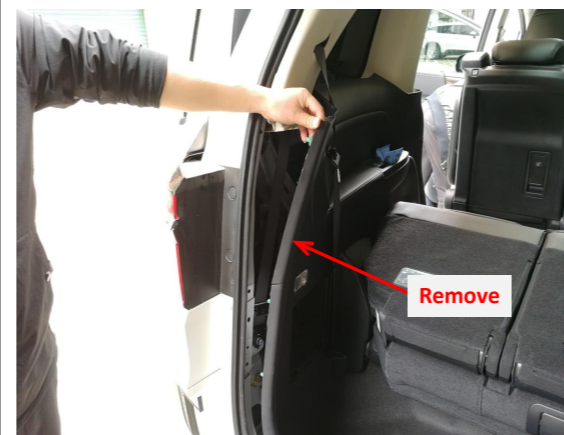
4. Remove the trim panel from the left side of the trunk to allow wiring harnesses to pass through.
