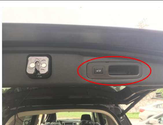
27. Install all the trim panels back and install the added tailgate switch.
