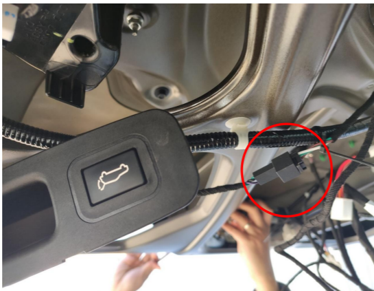
8. Connect the plug of the lock signal harness with the added tailgate switch
