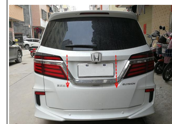
26. Press the added tailgate switch button to close the tailgate and test each function of the electric tailgate.
