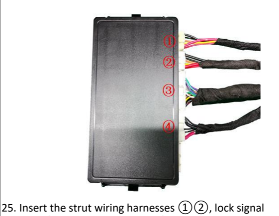
25. Insert the strut wiring harnesses ①②, lock signal harness ③, and power harness ④ into the ECU in sequence.
