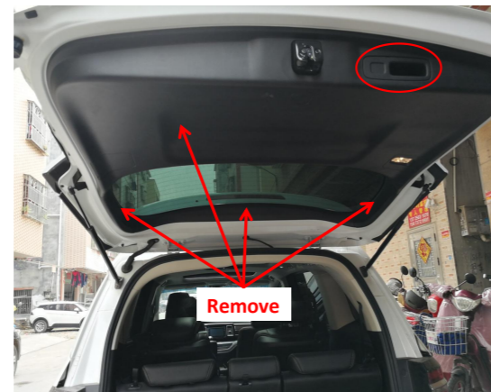
3. Remove the tailgate trim panels.
