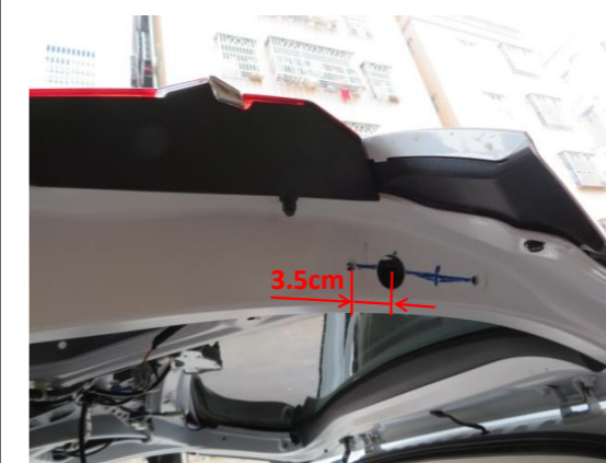
10. Remove the tailgate bracket and drill a hole at its position with a \phi 21 drill bit. Both sides are the same.
