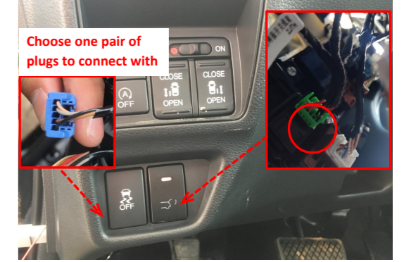
21. Install the added front switch and connect the plugs for backlight (due to configuration differences, two pairs of plugs have been reserved. Choose the correct one pair for connection and pay attention to avoid the plug of multifunctional combination button).
