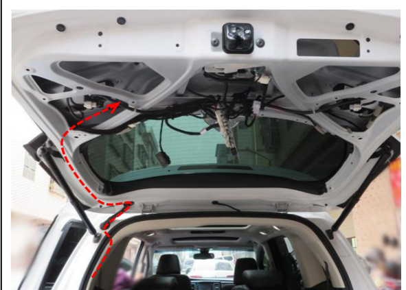
16. Route the power harness to the tailgate.
