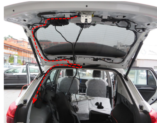
8. Route the lock signal harness to the left side of the trunk (do not connect plugs before inserting terminals into
