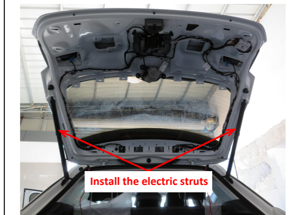
16. Install the electric struts, L on the left and R on the right (the first letter of the strut code).
