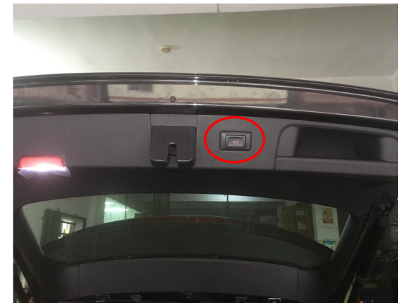
26. Install the added tailgate switch and reinstall all the trim panels.
