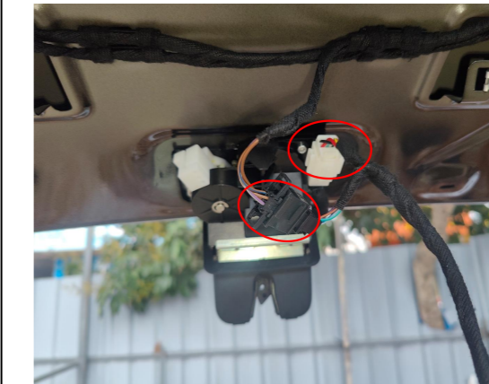
10. Connect the plugs of the lock signal harness to the plugs of the power latch.
