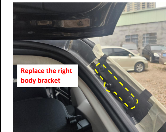
15. Replace the right body bracket (use original screws).
