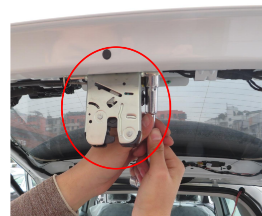
7. Remove the original latch and install the power latch.
