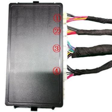
24. Insert the left and right strut wiring harnesses ① ②, lock signal harness ③, and power harness ④ into the ECU in sequence.
