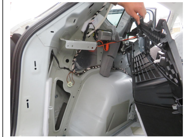
6. Remove the trim panel on the left side of the trunk.
