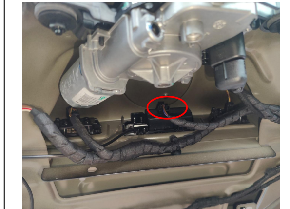
11. Connect the plugs of the lock signal harness to the plugs of original tailgate switch.
