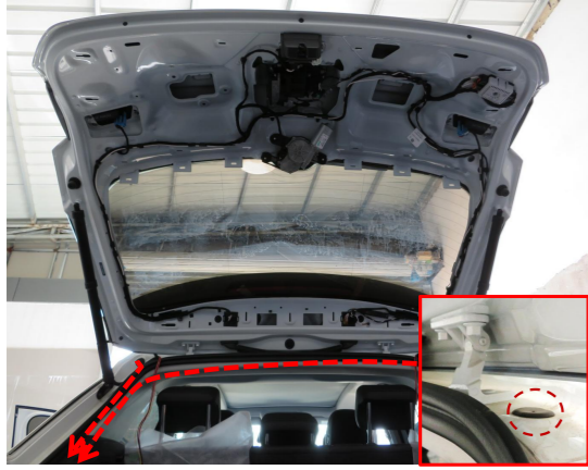
17. Remove the rubber plug beside the hinge and route the strut wiring harness to the left side of the trunk.
