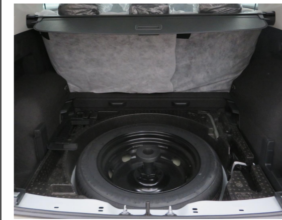
5. Take out the trunk floor mat and remove the lower trunk trim panel.
