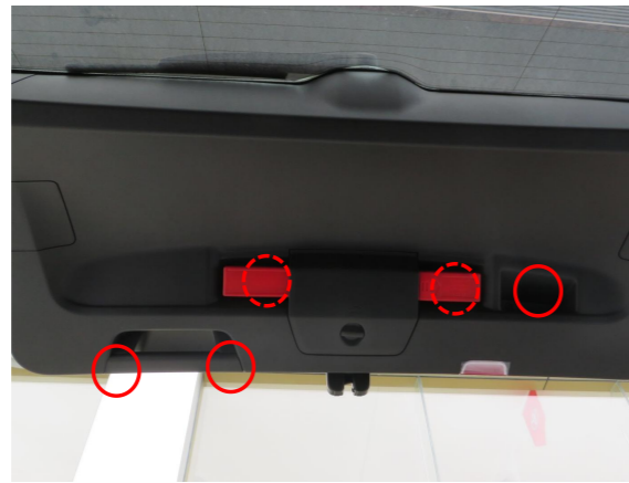
3. Remove the screws from the tailgate trim panels.
