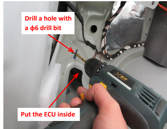
23. Drill a hole at the indicated position with a \phi 6 drill bit for installing the ECU bracket.
