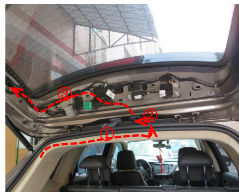
12. Thread the power harness to the tailgate (no plug connection before inserting terminals into the wiring harness connector).
