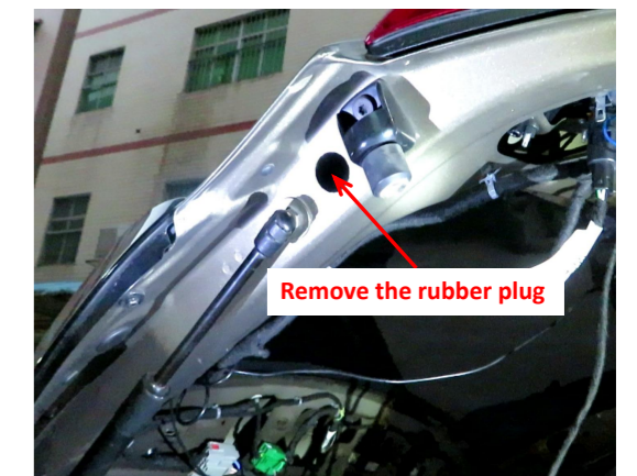
6. Remove the waterproof rubber plug from the left side of the tailgate.
