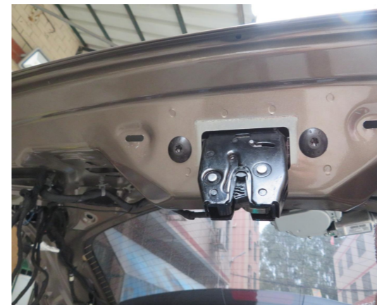
4. Remove the original latch and install our power latch.
