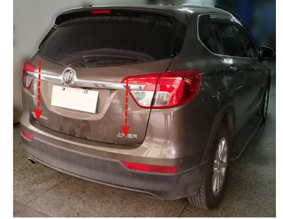
21. Initialize the system once and test each function of the electric tailgate.
