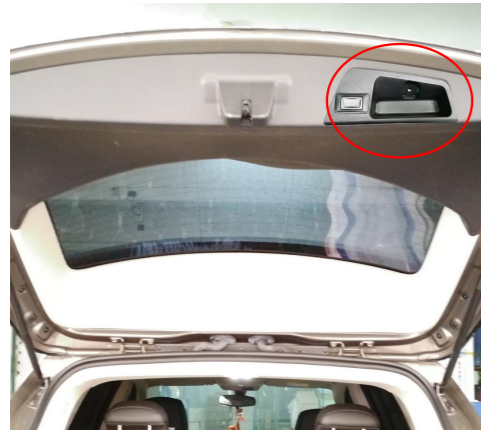
22. Reinstall all trim panel and install the added tailgate switch.
