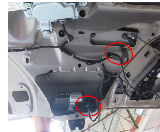
5. Connect the lock signal harness with the plugs of the power latch and the added tailgate switch.
