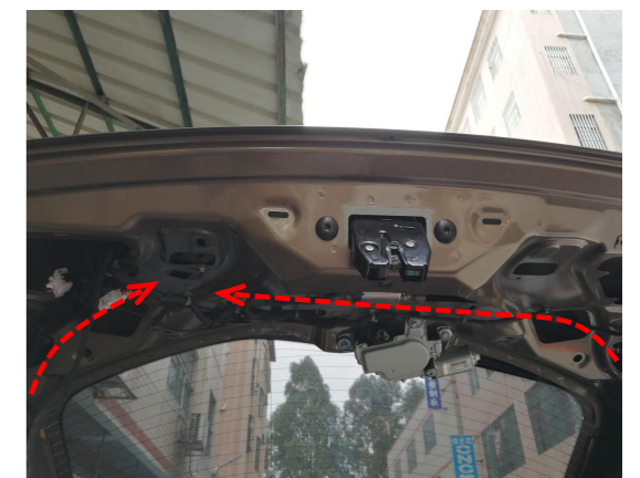
11. Route the strut wiring harnesses as indicated in the diagram.
