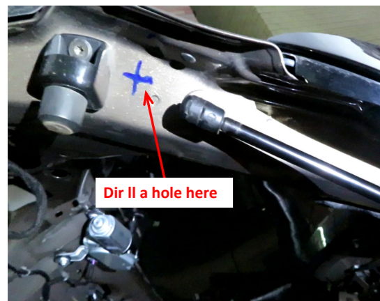
7. Drill a hole at the indicated position with a \phi 22 mm drill bit on the right side of the tailgate .
