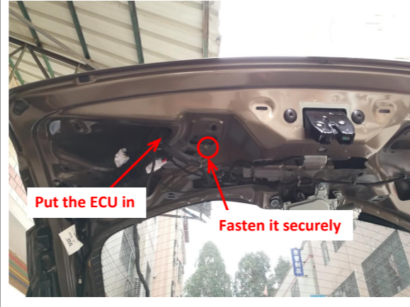
19. Remove the original fastener for the installation of the ECU bracket. Put the ECU in Fasten it securely
