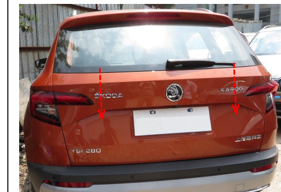
25. Press the added tailgate switch to open and close the tailgate once for initializing the system, and then test the functions of the electric tailgate.
