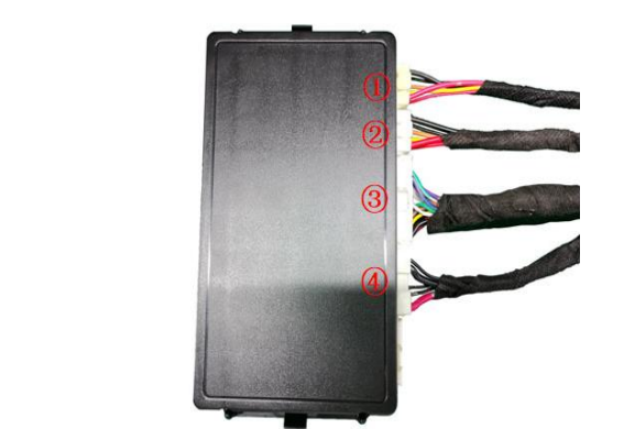
24. Insert the strut wiring harnesses ①②, lock signal harness ③, and power harness ④ into the ECU in sequence.
