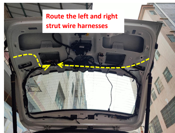
8. Thread the left and right strut wiring harnesses into the tailgate through the drilled holes.
