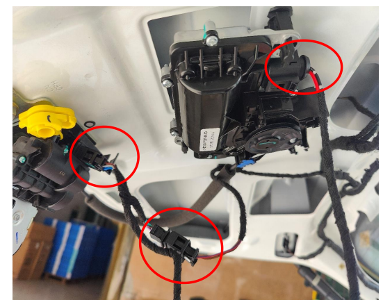
13. Connect the lock signal harness to the plugs of the lock latch and the actuator.
