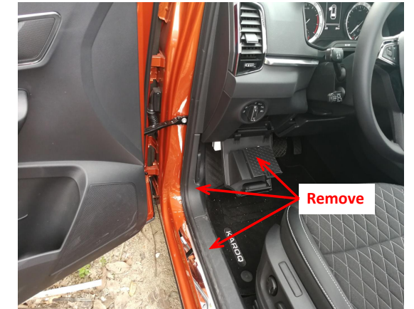
1. Remove the front left side trim panel, door sill panel and the storage box.
