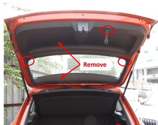
3. Remove the tailgate trim panels.
