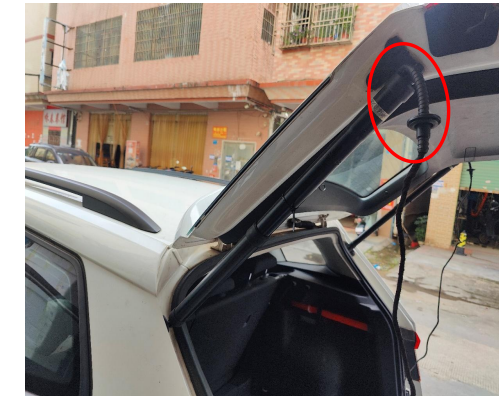
5. Install the electric struts, L on the left and R on the right (the first letter of the strut code), making sure the ends with wiring harnesses are on the tailgate.
