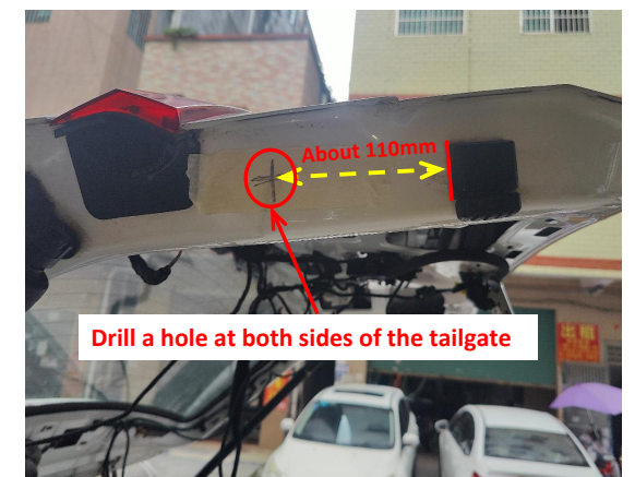
6. Mark the positions to be drilled with tape and pay attention to avoid the taillights.
