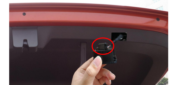
27. Reinstall all trim panels and install the added tailgate switch.
