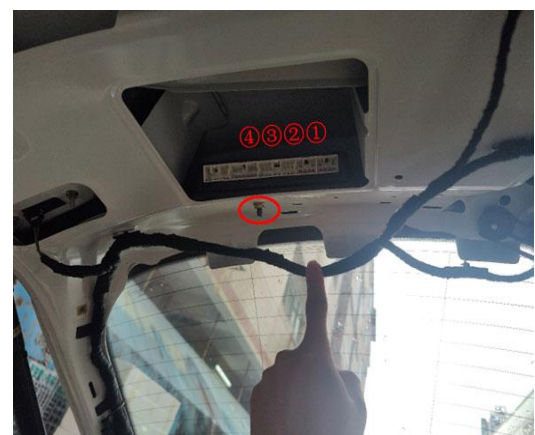
23. Place the ECU at the indicated position and secure it with a nut.
