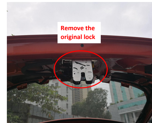
10. Remove the original latch.
