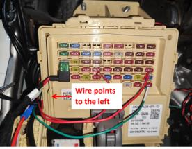
24. Plug the fuse tap into the fuse box and pay attention to the direction of wire.
