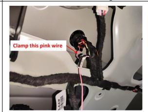
15. Clamp the indicated pink wire of the original tailgate switch plug to connect it to the pink wire of lock signal harness. | harness in the same way)
