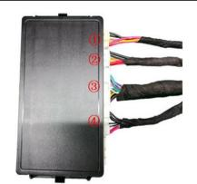
27. Insert the left and right strut wiring harnesses (1)(2), lock signal harness 3, and power harness 4 into the ECU in sequence.
