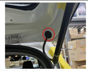
10. Thread the left and right strut wiring harnesses through the indicated hole on both sides into the tailgate.
