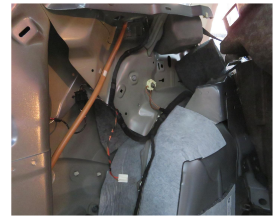
6. Remove the trim panel on the left side of the trunk.
