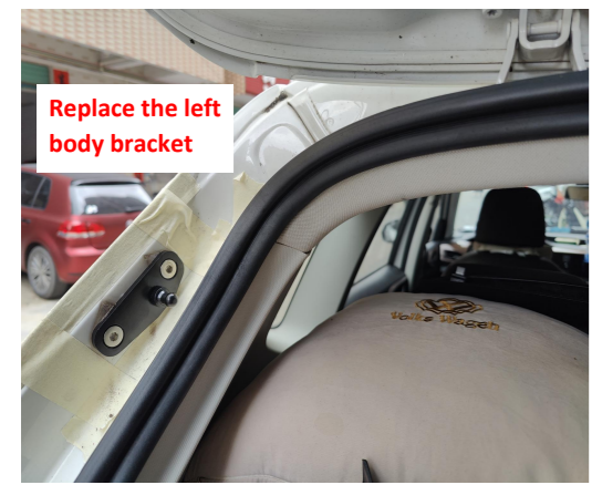
12. Replace the left body bracket and make sure the ball stud is positioned closer to the inner side.
