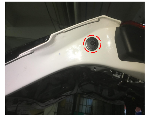
11. Replace the ball studs on both sides of the tailgate.
