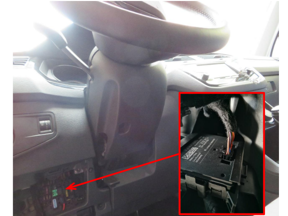
21. Find out the CAN box behind the fuse box and connect to the indicated plug and its socket.
