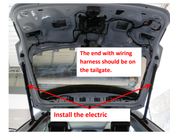
15. Install the electric struts, L on the left and R on the right (the first letter of the strut code).
