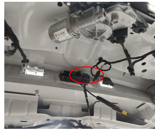
9. Connect the plugs of the lock signal harness to the plugs of original tailgate switch.
