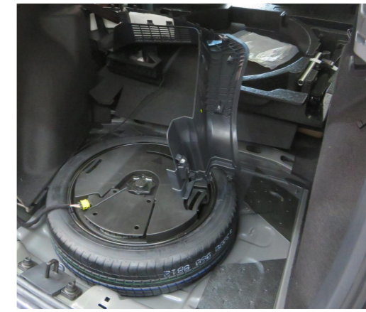
5. Take out the trunk floor mat and remove the lower trim panel.
