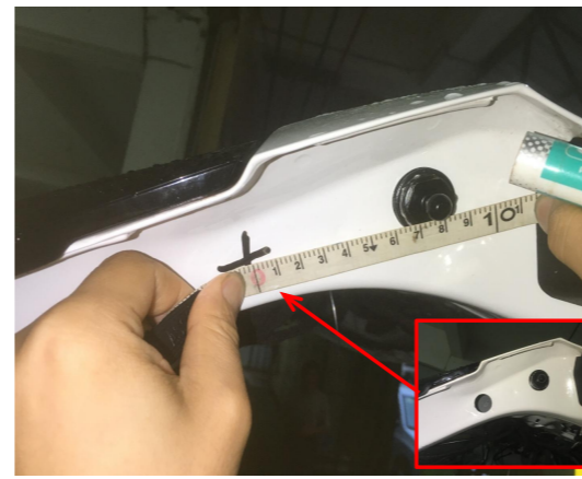
14. Drill a hole at the indicated position with a 14mm drill bit.
