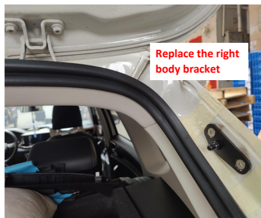
13. Replace the right body bracket and make sure the ball stud is positioned closer to the inner side.
