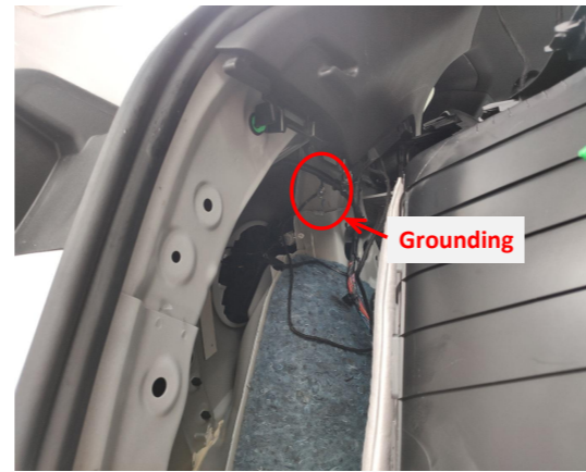
19. Ground at the left side of the trunk.
