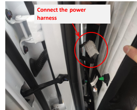
20. Connect the power harness to the B-pillar plugs at rear left B-pillar.
