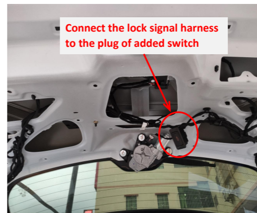
15. Connect the lock signal harness to the plug of the added tailgate switch.
