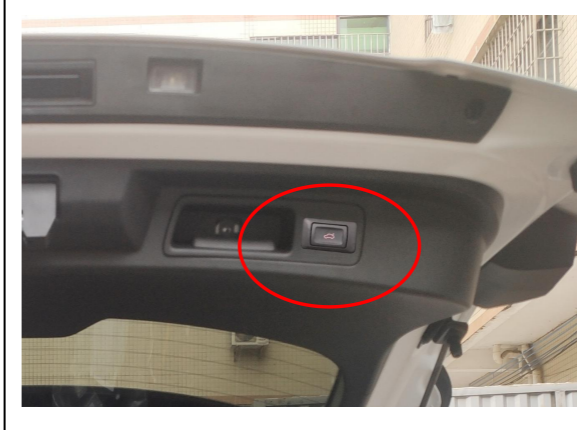
30. Reinstall all trim panels and install the added tailgate switch.
