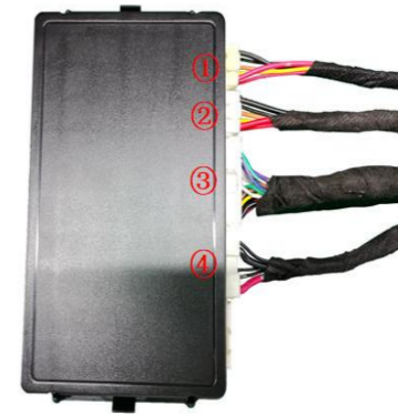
25. Insert the strut wiring harnesses ①②, lock signal harness ③, and power harness ④ into the ECU in sequence and then mount it onto its bracket.
