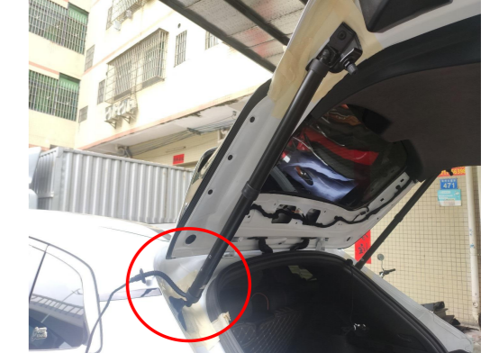
6. Install the electric struts, L on the left and R on the right (the first letter of the strut code), making sure the ends with wiring harnesses are on the vehicle body.
