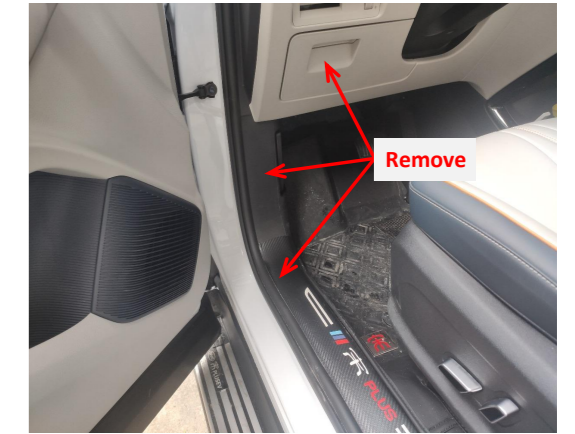
1. Remove the front left side trim panel, door sill panel and storage box.
