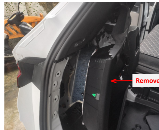
4. Remove the trunk floor mat, foam storage box and the left side trim panel.
