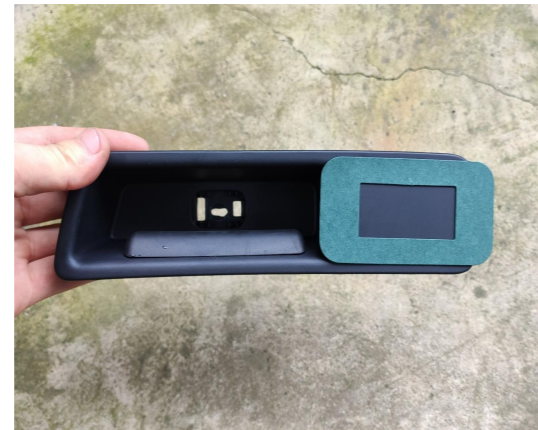
28. Stick the hole template to the tailgate handle and open a hole for the installation of added tailgate switch.
