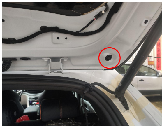
7. Thread the strut wiring harness through the indicated hole into the tailgate. Both sides are the same.
