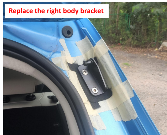
7. Replace the right body bracket.
