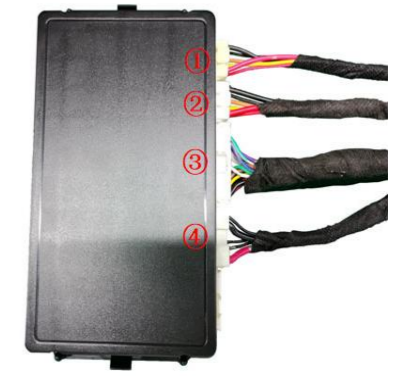
26. Insert the strut wiring harnesses ①②, lock signal harness ③, and power harness ④ into the ECU in sequence.
