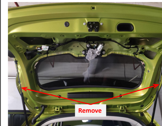
5. Remove the original gas struts.
