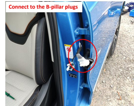
20. Connect the power harness to the B-pillar plugs at the rear left side B-pillar.
