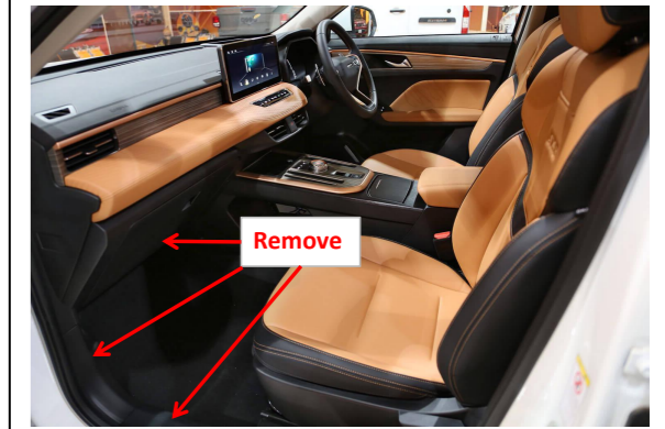
1. Remove the front left side door sill panel and storage box.
