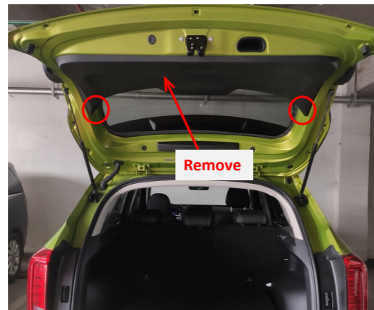
3. Remove the tailgate trim panel.
