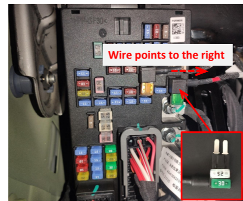
24. Move the fuse from the fuse box to the fuse tap and then plug the fuse tap into the fuse box. Pay attention to the direction.
