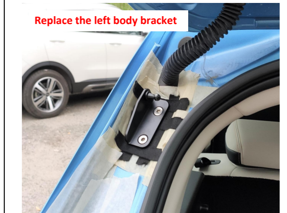
6. Replace the left body bracket
