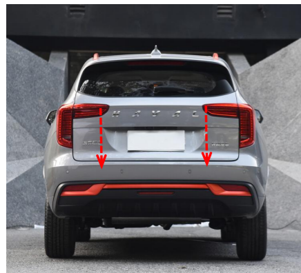
27. Press the added tailgate switch button to open and close the tailgate once for initializing the system, and then test each function of the electric tailgate.
