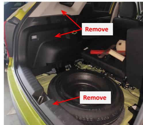
4. Take out the floor mat and foam storage box from the trunk. Remove the left side trim panel and door sill panel.
