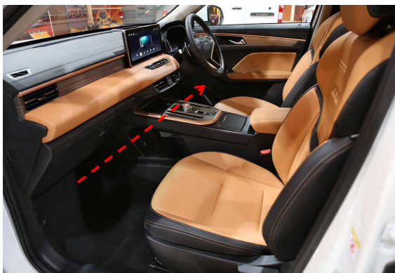
22. Locate the fuse box. If the fuse box is located at the driver's area, thread the the fuse tap from the front passenger side to the driver side.
