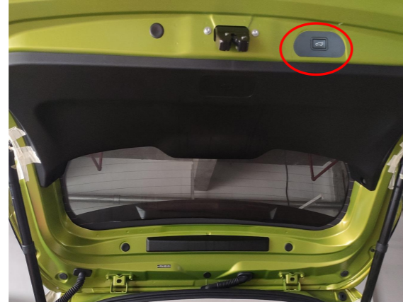
28. Reinstall all trim panels and install the added tailgate switch (remove the original small cover panel).
