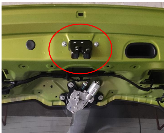
12. Remove the original latch and install the power latch.
