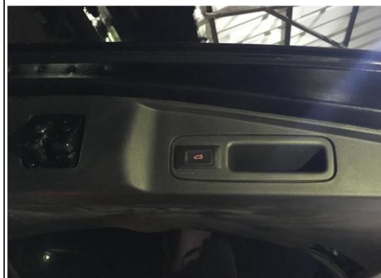
30. Install all the trim panels back and install the added tailgate switch.
