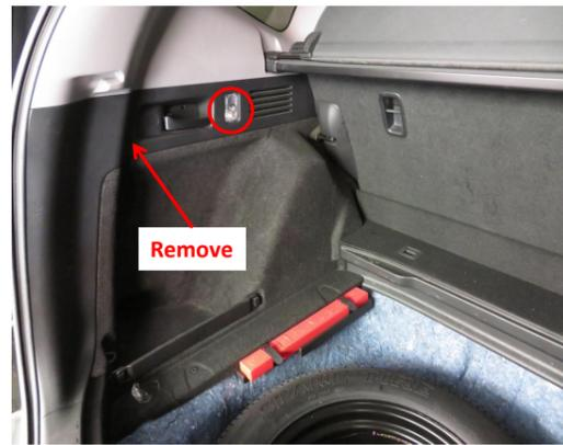
3. Take out the trunk floor mat and remove the trim panel on the left side of the trunk.
