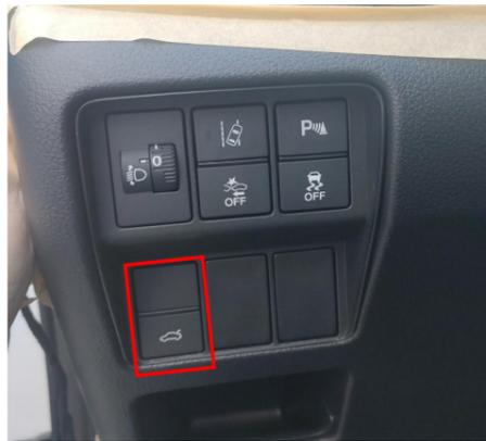
22. Remove the blank button and install the added front switch button.
