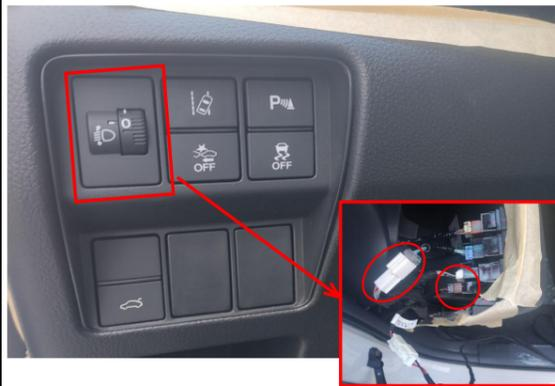
23. Connect the power harness to the plugs of the front switch behind the panel.
