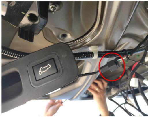
17. Connect the plug of the lock signal harness to the plug of the added tailgate switch.
