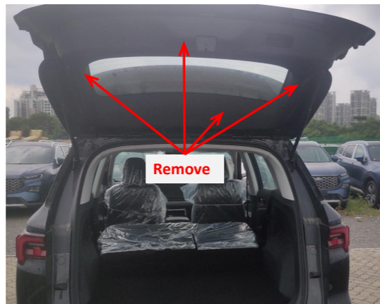
3. Remove the tailgate trim panel.
