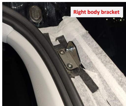
7. Replace the right body bracket.
