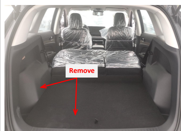
4. Take out the trunk floor mat and the trim panel on the left side to allow the wiring harnesses to pass through.
