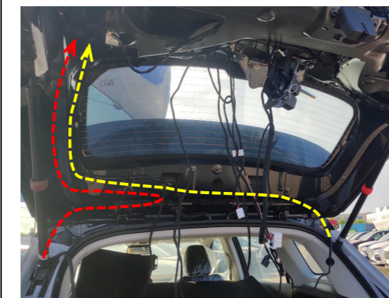
10. Route the strut wiring harnesses to the tailgate as shown above.
