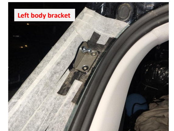
6. Replace the left body bracket.
