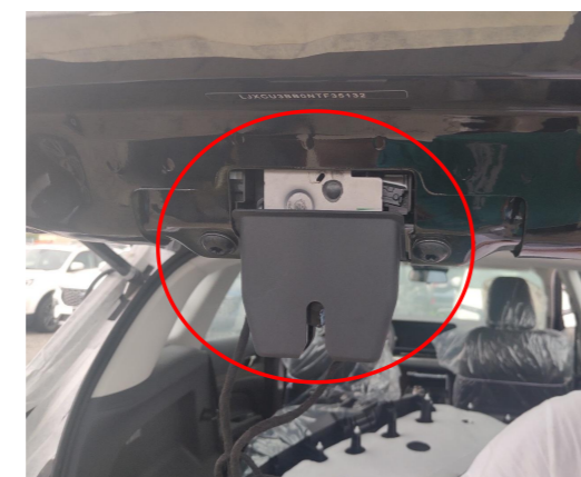
13. Remove the original latch.
