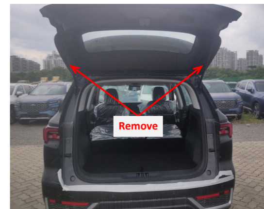
5. Remove the original gas struts.
