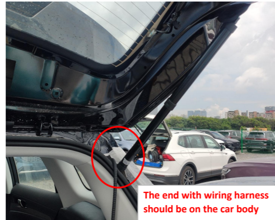
8. Install the electric struts, L on the left and R on the right (the first letter of the strut code).
