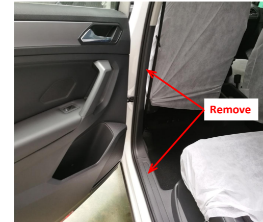
5. Remove the rear left side door sill panel and B-pillar trim panel.
