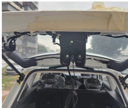
9. Install the power latch.
