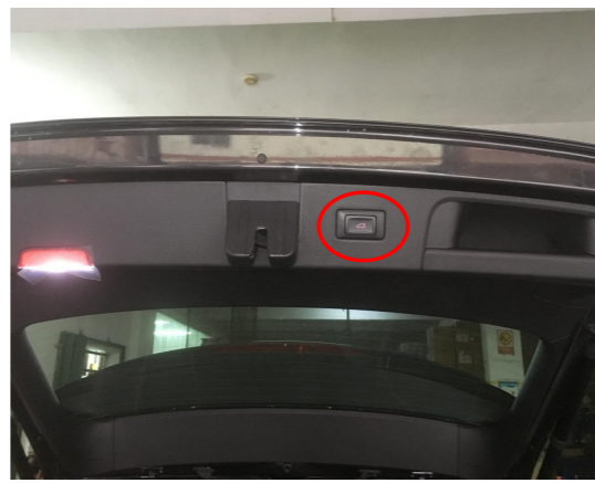
24. Reinstall all trim panels and install the added tailgate switch.
