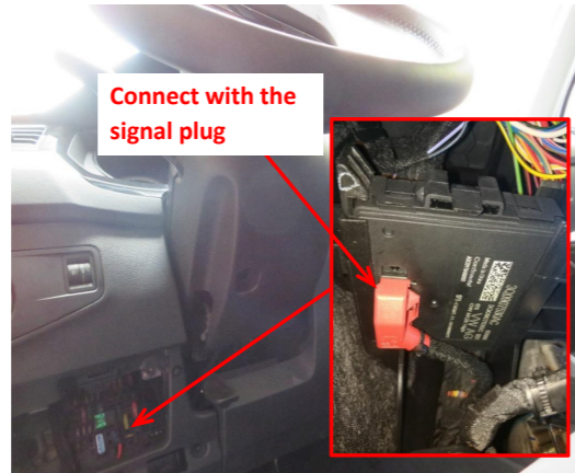
18. Connect the power harness to the indicated signal plug and its socket on the CAN box behind the fuse box.
