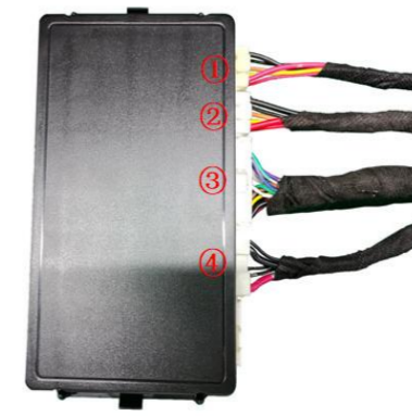
20. Insert the strut wire harnesses ① ②, lock signal harness ③, and power harness ④ into the ECU in sequence and then mount the ECU onto its bracket.
