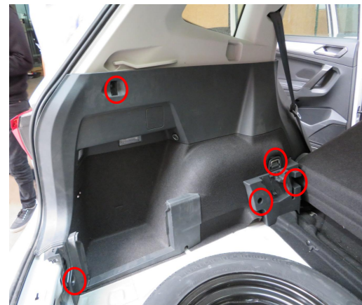
2. Take out the trunk floor mat. Remove the screws from door sill panel and the trim panel on the left side.
