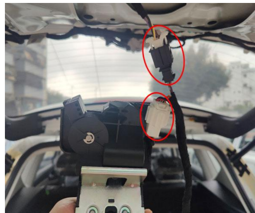
7. Connect the plugs of the lock signal harness to the power latch.
