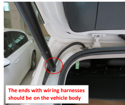
14. Install the electric struts, L on the left and R on the right (the first letter of the strut code),
