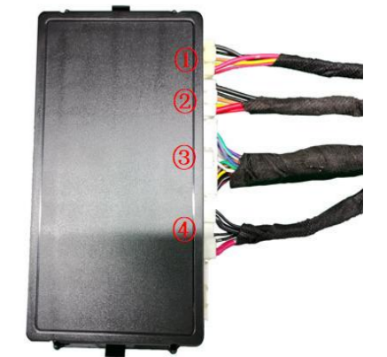
31. Insert the strut wiring harnesses ①②, lock signal harness ③, and power harness ④ into the ECU in sequence.
