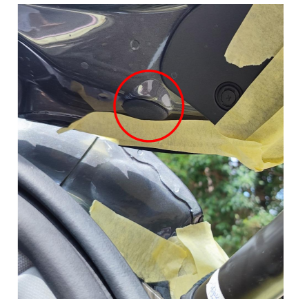
11. Remove the indicated rubber plug and thread the strut wiring harnesses through the hole into the tailgate.
