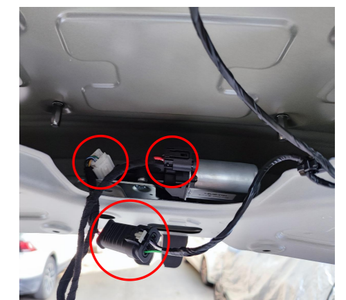
16. Connect the plugs of the lock signal harness to the power latch.
