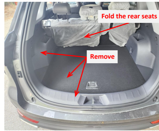
4. Take out the trunk floor mat and foam storage box, remove the door sill panel and the panel on the left side of
