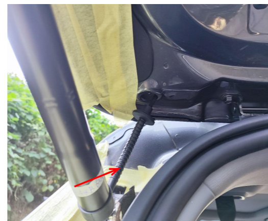
14. Leave a certain length of tube outside to prevent strut wiring harness from being pulled, the same on both sides.
