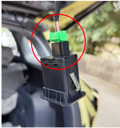
17. Connect the plug of lock signal harness to the added tailgate switch.
