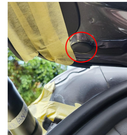
10. Remove the indicated rubber plug and thread the strut wiring harnesses through the hole into the tailgate.
