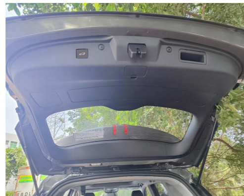
33. Reinstall all the trim panels and install the added tailgate switch.
