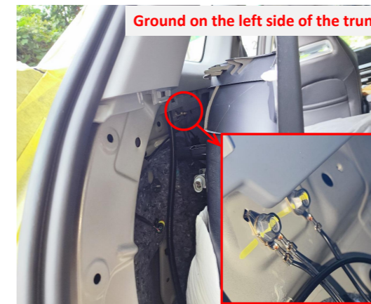
25. Ground at the indicated position on the left side of the trunk.
