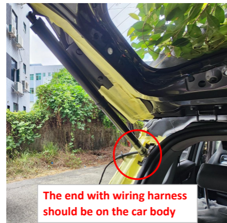
8. Install the left electric struts, L on the left and R on the right (the first letter of the strut code).
