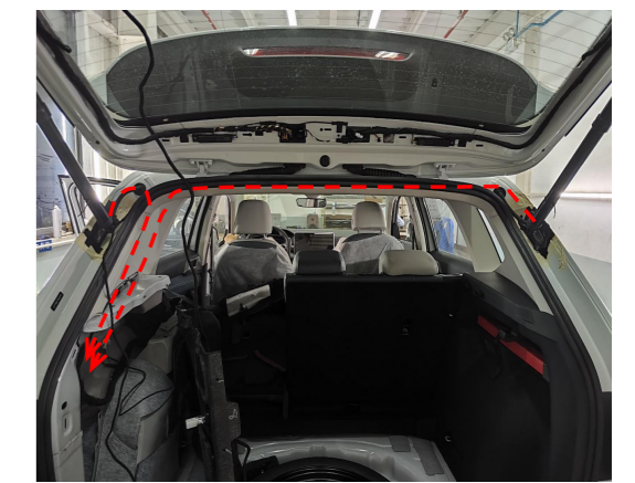
11. Route the left and right strut wiring harnesses to the left side of the trunk.
