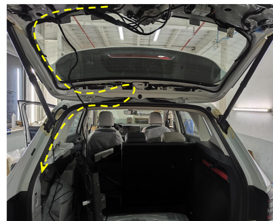
13. Route the lock signal harness to the left side of trunk along with original wiring harness.
