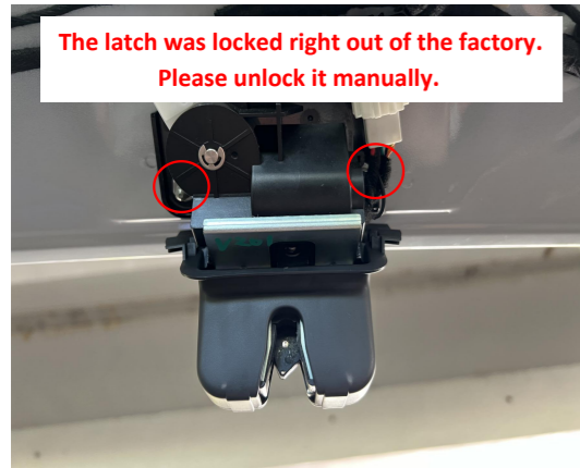
17. Install the power latch and cover the latch with original latch casing.
