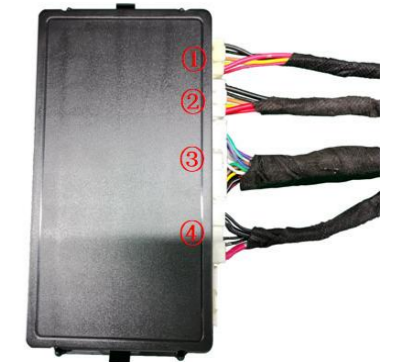
26. Insert the left and right strut wiring harnesses ①②, lock signal harness ③, and power harness ④ into the ECU in sequence.
