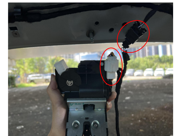
16. Connect the plugs of lock signal harness with the plugs of the power latch.
