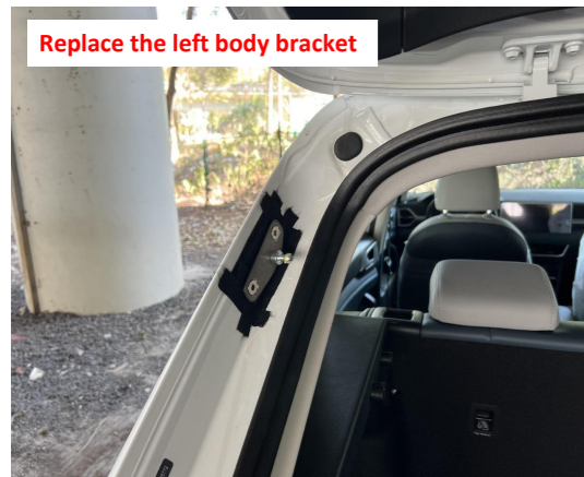
7. Replace the bracket on the left side of the trunk.
