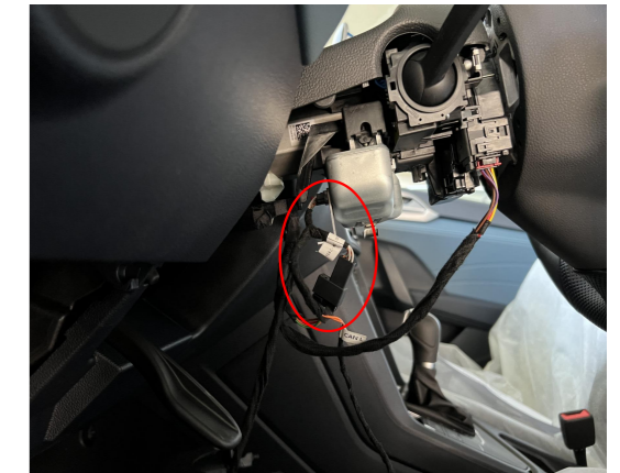
21. Connect the lock signal harness with CAN signal plugs inside the steering column panel.
