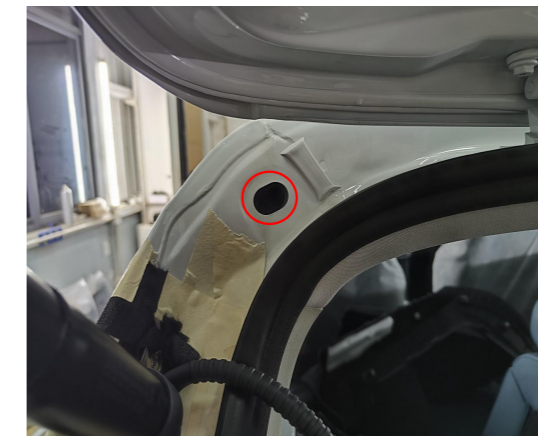
10. Thread the strut wiring harness through the indicated hole into the trunk.
