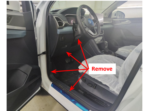
1. Remove front left door sill panels, switch panel and steering column panel.
