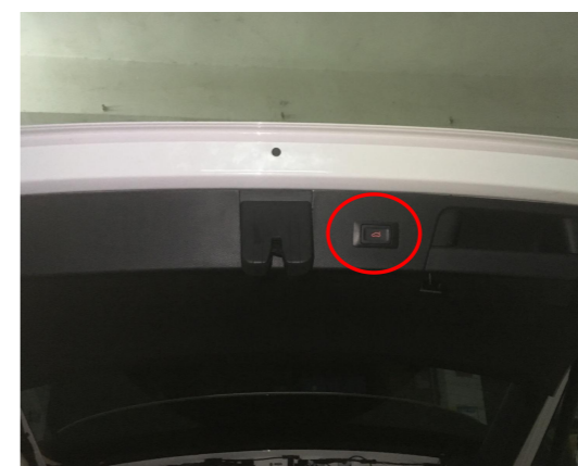
30. Install the added tailgate switch and reinstall all trim panels.
