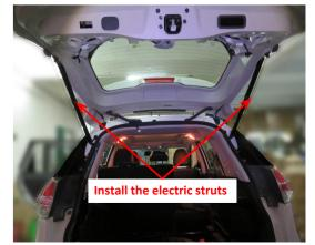
16. Install the electric struts, L on the left, R on the right (the first letter of the strut code).
