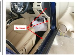
1. Remove the indicated triangular trim panel and door sill panels.
