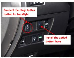
24. Install the added front switch and connect the plugs behind the panel for backlight.
