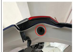
15. Replace the left and right sides ball studs and shims.
