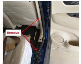
2. Remove the rear right door sill panel and B-pillar trim
