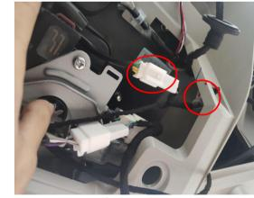
10. Connect the plugs of the lock signal harness to the plugs | 11. Connect the plugs of the lock signal harness to the plugs of the original tailgate switch.
