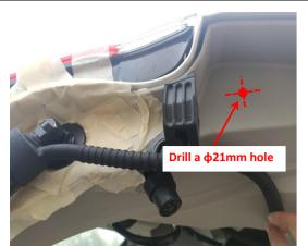
bit to allow the strut wiring harness to pass through.
