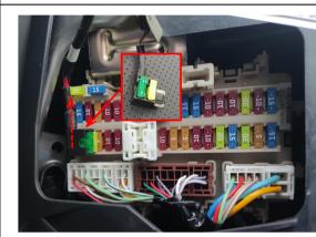
26. Move the fuse from from the fuse box to the fuse tap and then plug the fuse tap into the fuse box. Pay attention to the direction.
