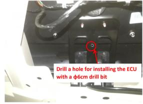
7.Drill a hole at the indicated bracket behind the latch position for installing the ECU (just need to drill through the bracket).
