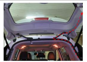
19. Route the power harness to the tailgate (do not connect the power before inserting terminals into the wiring harness 20. Insert the power harness terminals into the wiring connector).
