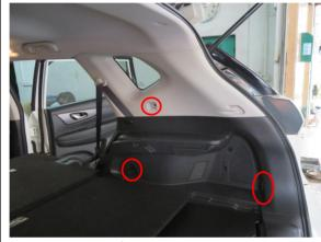
3. Take out the trunk floor mat and remove the screws in the circles from the rght side trim panel.
