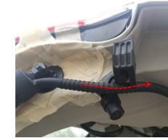
18. Pass the strut wiring harness through the shown 17. Drill a hole at the indicated position using a \$\phi 21mm drill position and the drilled hole into the tailgate and then plug the hole with hole plug.
