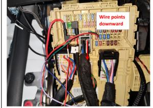
24. Plug the fuse tap into the fuse box and pay attention to the direction.
