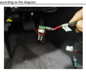
23. Move the fuse from the fuse box to the fuse tap.
