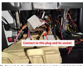
21. Connect to the CAN signal plug and its socket behind the fuse box.
