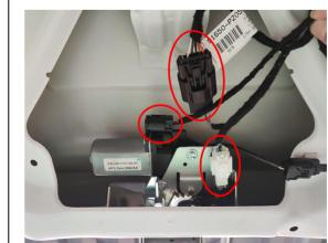
15. Connect the plugs of the lock signal harness to the plugs of the power latch and original latch.
