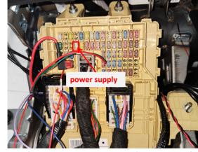
22. The fuse box is located at the driver's area and the fuse slot for power supply is indicated above.
