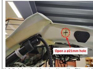
11. Drill a hole at the indicated position with a Ø21mm drill bit , the same on both sides.
