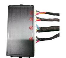
26. Insert the left and right strut wiring harnesses ①②, lock signal harness ③, and power harness ④ into the ECU in sequence.
