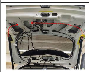
12. Therad the strut wiring harnesses into the tailgate.
