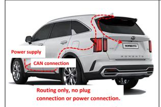
17. Route the power harness as indicated (if you need to install the added front switch, route the switch wiring harness in the same way).
