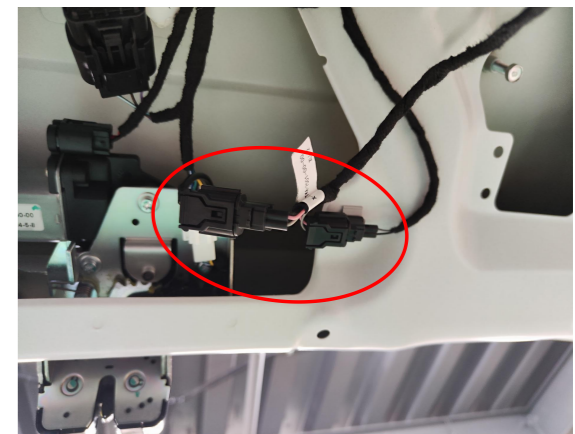
16. Connect the plugs of the lock signal harness to the plugs of original tailgate switch.
