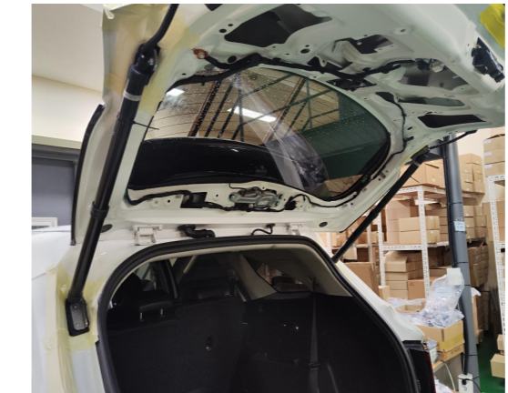
10. Install the electric struts, L on the left and R on the right (the first letter of the strut code).
