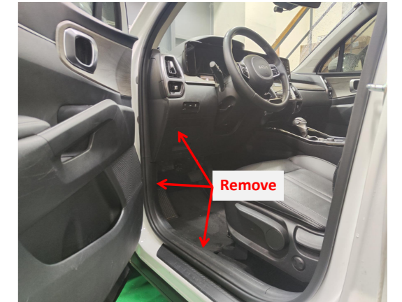
1. Remove the front left door sill panels and the fuse box trim panel.
