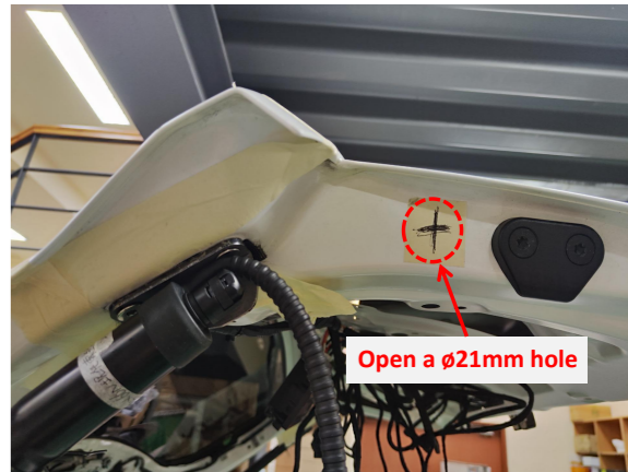
11. Drill a hole at the indicated position with a 21mm drill bit, the same on both sides.
