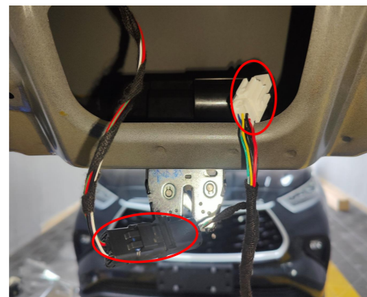
13. Connect the plugs of the lock signal harness to the plugs of the power latch.
