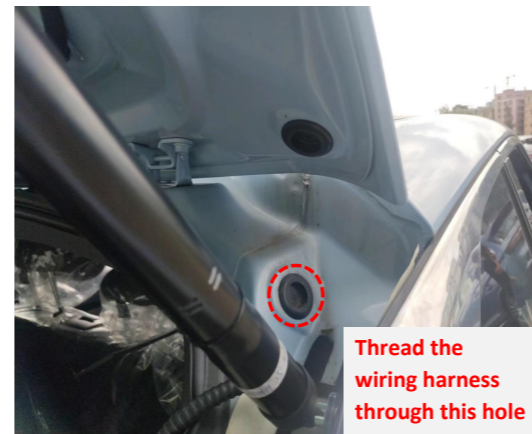
9. Thread the strut wiring harnesses through the indicated hole on both sides.
