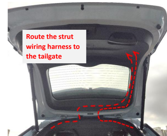
10. Route the strut wiring harness to the tailgate (routing first, then insert the terminals into the connector).
