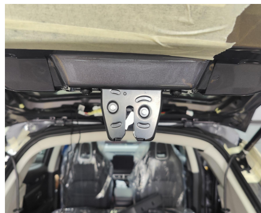
12. Remove the original latch, install the power latch with original screws and adjust the latch to the locked state.
