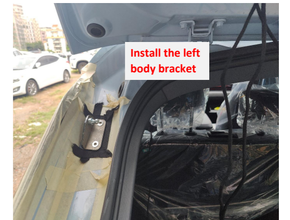
6. Replace the left body bracket and pay attention to the direction.
