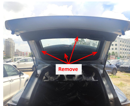
3. Remove the tailgate trim panels.
