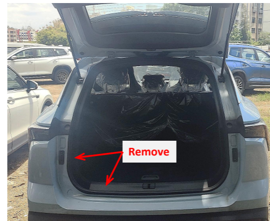
4. Remove the indicated trunk trim panels.
