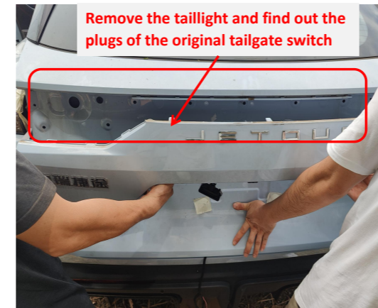
14. Remove the taillight and find out the plugs of the original tailgate switch
