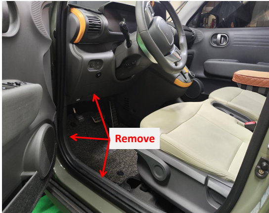
1. Remove the front left door sill panels and the fuse box trim panel.
