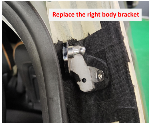
6. Replace the right body bracket.
