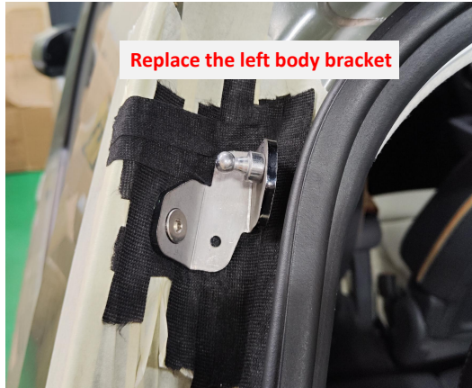
5. Replace the left body bracket.
