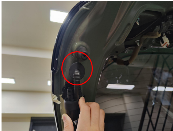
10. Plug the hole securely.
