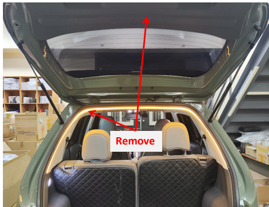
3. Remove the tailgate trim panels.
