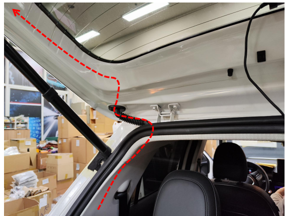
15. Thread the power harness to the tailgate.
