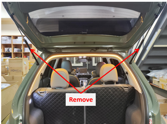
4. Remove the original gas struts.
