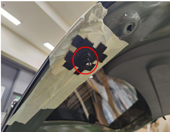
7. Replace the ball studs on both sides.
