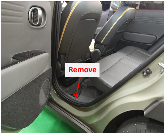
2. Remove the rear left door sill panel.
