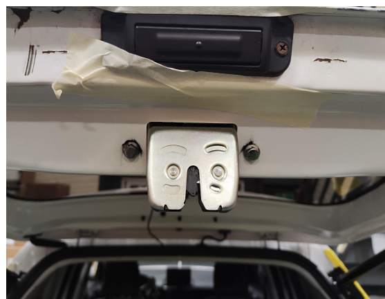
11. Remove the original latch.
