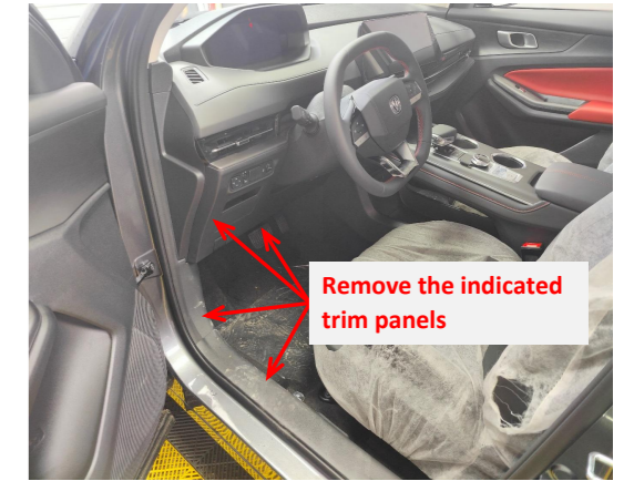
1. Remove the indicated trim panels.
