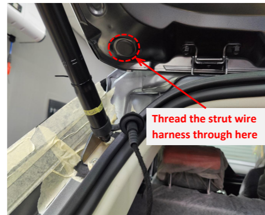
9. Remove the indicated rubber plug and thread the strut wiring harness through the hole into the tailgate.
