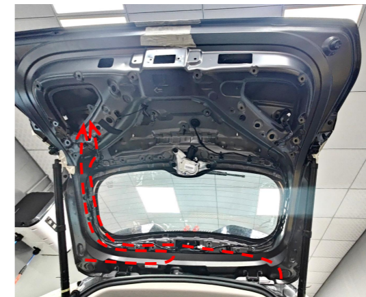
10. Route the left and right strut wiring harnesses as indicated above.
