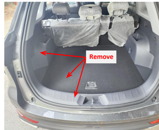
4. Remove the indicated trunk floor mat, door sill trim and the trim panel on the left side.
