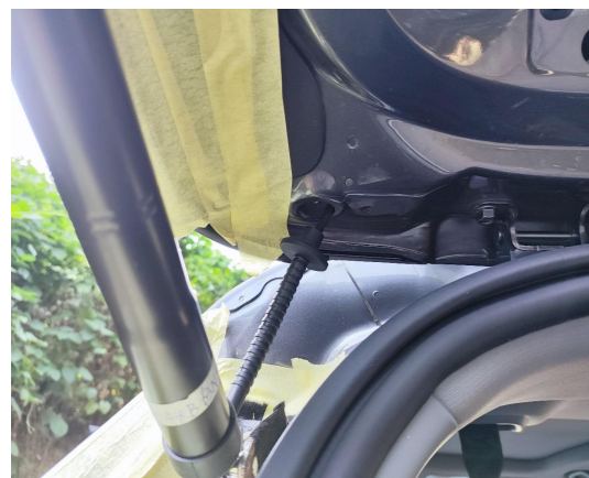
12. Leave a certain length of tube outside to prevent strut wiring harness from being bent, the same on both sides.
