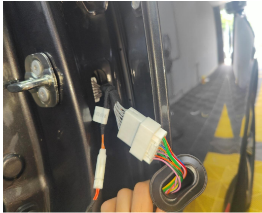
22. Connect the signal plugs of the power harness with the B-pillar signal plugs.
