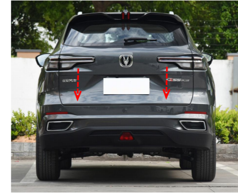
30. Manually close the tailgate to the position where it touches the lock striker and press the added tailgate switch button. After finishing the system initialization, test each function of the electric tailgate.
