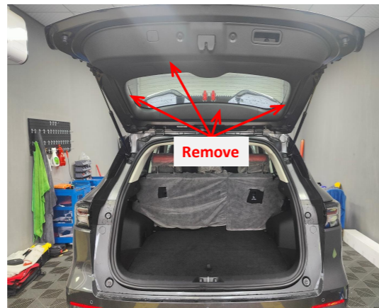
3. Remove the tailgate trim panels.
