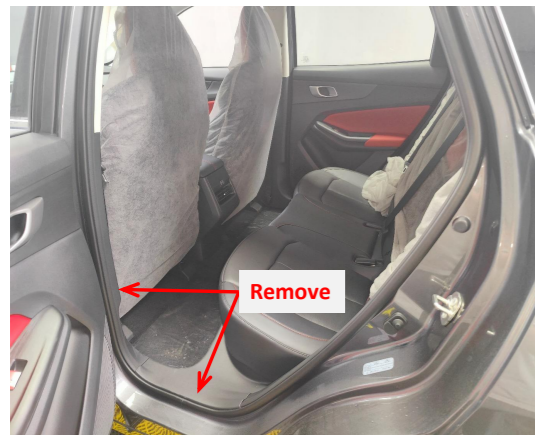
2. Remove the rear left side door sill panel and B-pillar trim panel.
