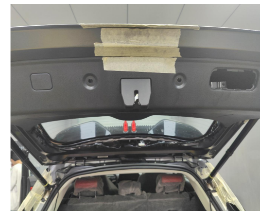
15. Install the power latch with original screws.
