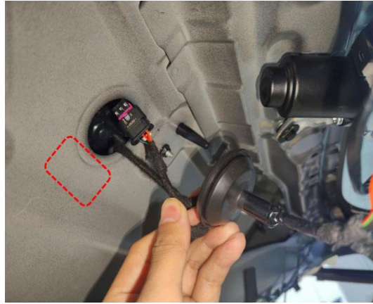
17. Take out the handle switch plug from the indicated location and connect with the plugs of lock signal harness.
