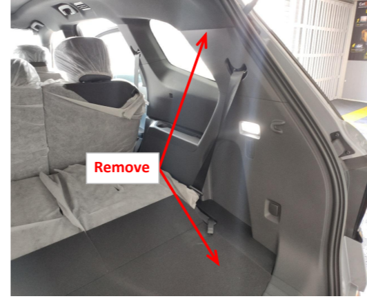
4. Remove the trunk floor mat and the trim panel on the right side of the trunk.
