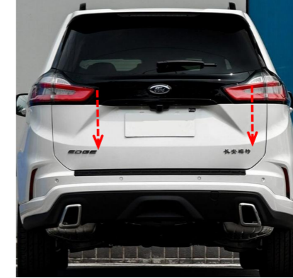
25. Press the added switch on the tailgate to open and close the tailgate once for initializing the system, and then test each function of the electric tailgate.
