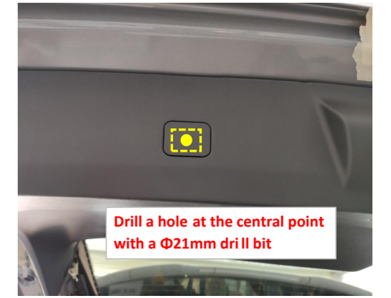
26. Mark the central point of the small panel and drill a hole with a \phi 21\text{mm} drill bit.
