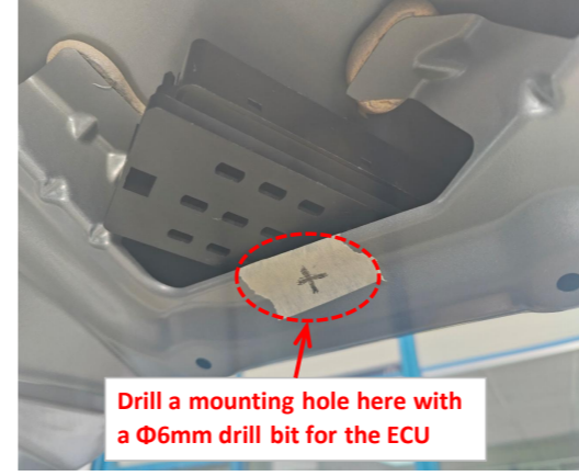
24. Stick the hole template to the marked position and drill a mounting hole for the ECU with a \phi 6\text{mm} drill bit.
