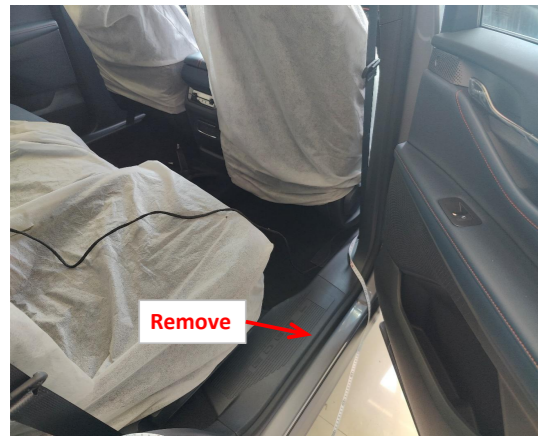
2. Remove the rear right side door sill panel.
