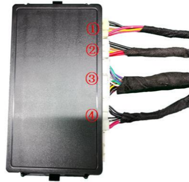
23. Insert the strut wiring harnesses ①②, lock signal harness ③, and power harness ④ into the ECU in sequence.
