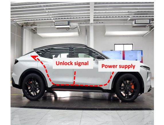
16. Route the power harness (do not connect plugs before inserting terminals into wiring harness connector).
