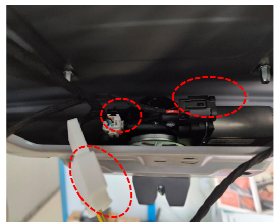
13. Connect the three plugs of the lock signal harness to the plugs of the power latch.
