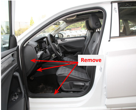
1. Remove the front left side door sill panel and the trim panels of the fuse box.
