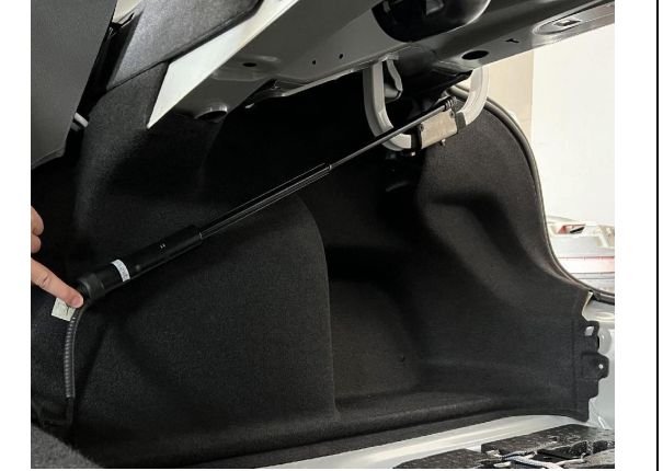
26. Install the electric struts, L on the left and R on the right (the first letter of the strut code).
