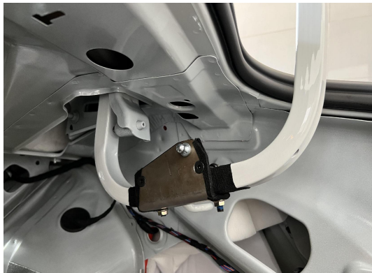
14. Tighten the nuts on those bolts.
