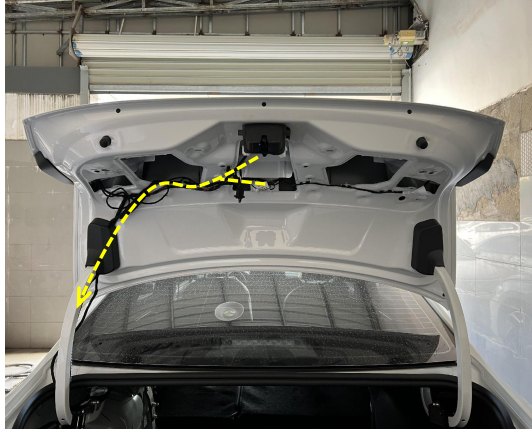
19. Route the lock signal harness to the left side of the trunk.
