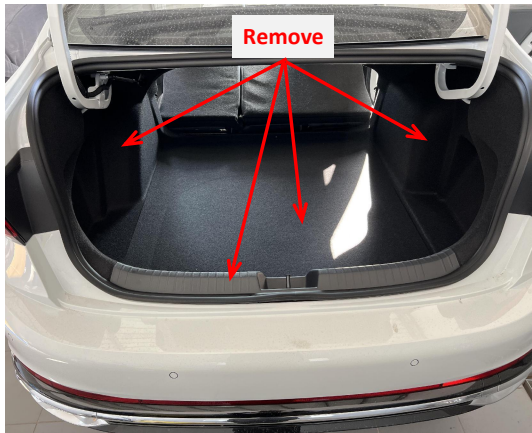
4. Take out the trunk floor mat and the indicated trim panels.
