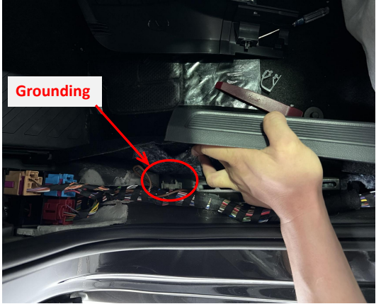
22. Ground at the left side of the driver's position.
