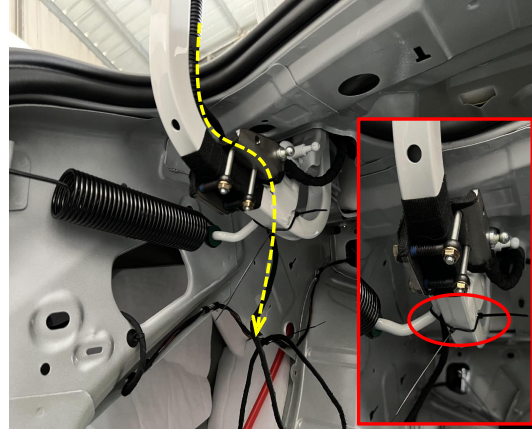
20. Tie the lock signal harness to the hinge as indicated and leave a certain length.
