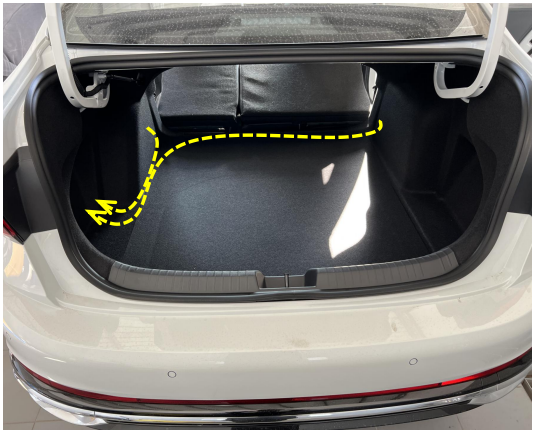
27. Route the strut wiring harnesses to the left side of the trunk.
