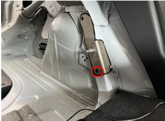
8. Secure the left body bracket at the indicated position first and insert the M10 bolt into the position① and make it out from the indicated position.
