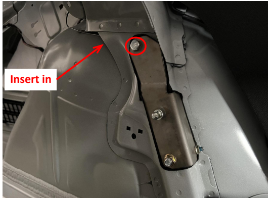
9. Insert the nut with handle into the indicated position and screw the nut onto the indicated bolt.
