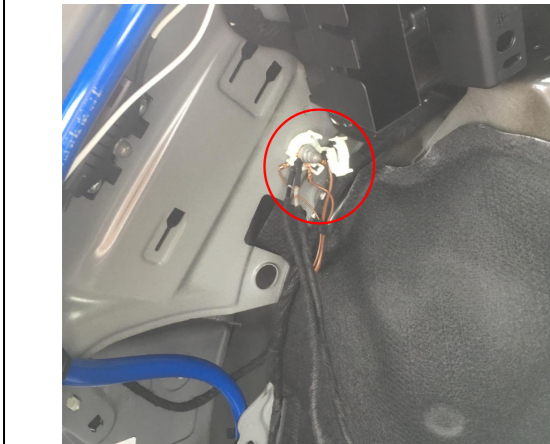
22. Ground at the left side of the trunk.
