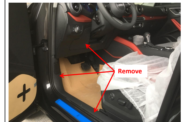
1. Remove the front left side trim panel, door sill panel and the storage box.
