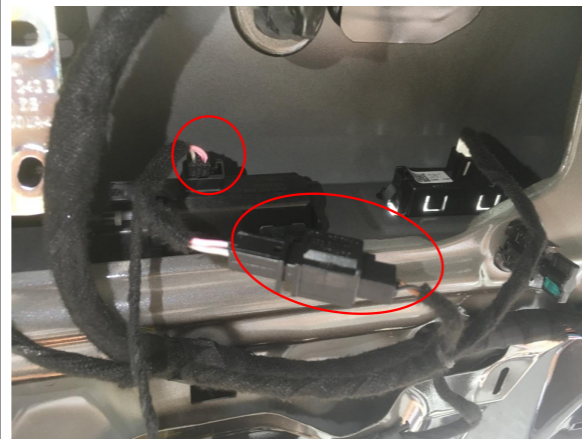
9. Connect the plugs of lock signal harness to the original tailgate switch.
