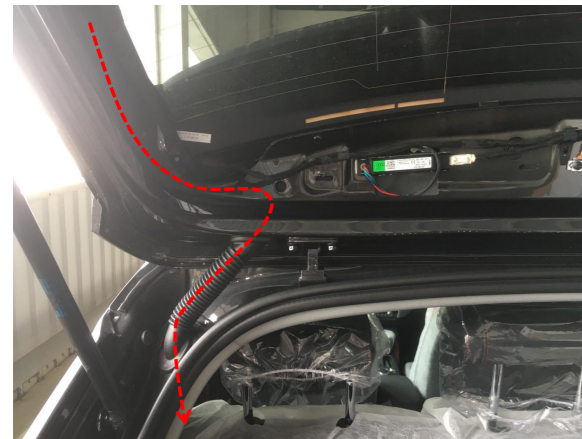
7. Route the lock signal harness to the left side of the trunk (do not connect plugs for now).
