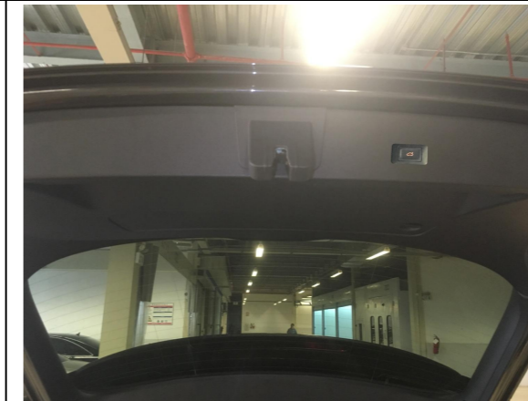
30. Reinstall all the trim panel and fit the added tailgate switch in.
