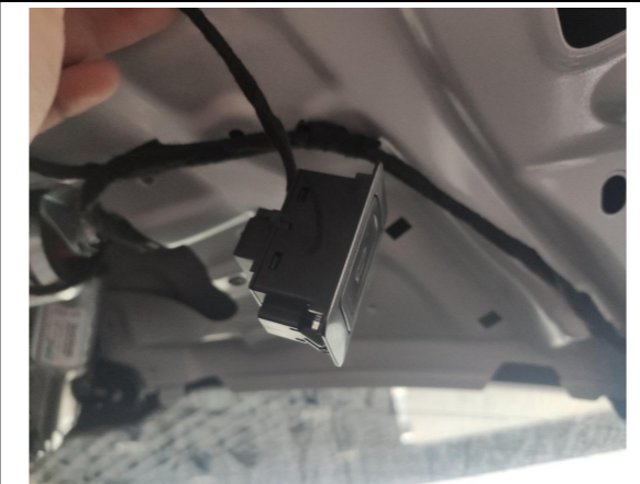
14. Connect the plug of lock signal harness with the added tailgate switch.
