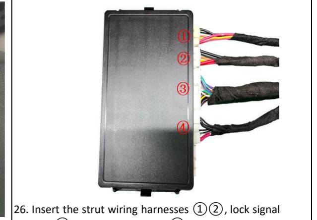
26. Insert the strut wiring harnesses ①②, lock signal harness ③, and power harness ④ into the ECU in sequence and mount the ECU onto its bracket.
