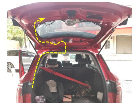
16. Route the power harness to the tailgate (routing only, no plug or power connection).
