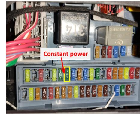
20. The fuse box is located behind the storage box at the driver's position and the fuse slot for power supply is indicated above.
