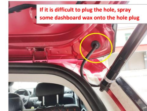
10. Plug the hole tightly. Leave a certain length of rubber tube outside and to prevent it from being pulled during the movement of tailgate.
