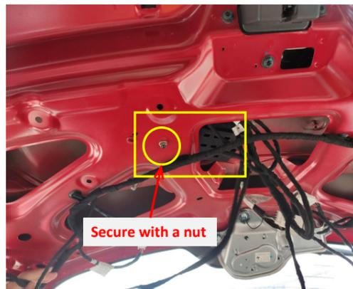
22. Place the ECU bracket at the indicated position and secure it with a nut.
