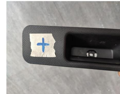
25. Stick the hole template to the marked position on the tailgate handle and open a hole for the added tailgate switch.
