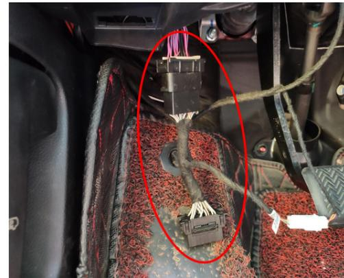
19. Connect one plug of the power harness to the OBD plug and place another plug in the slot of the OBD plug.
