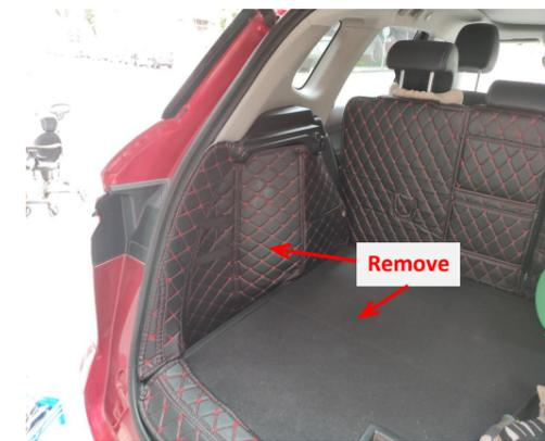
4. Remove the trunk floor mat and the trim panel on the left side of the trunk.
