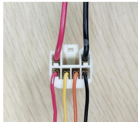
9. Insert the strut Wiring harness terminals into the Wiring harness connector as shown above.
