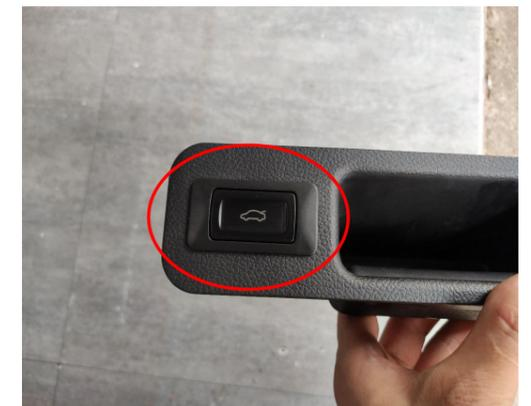
26. Install the added tailgate switch in the handle.
