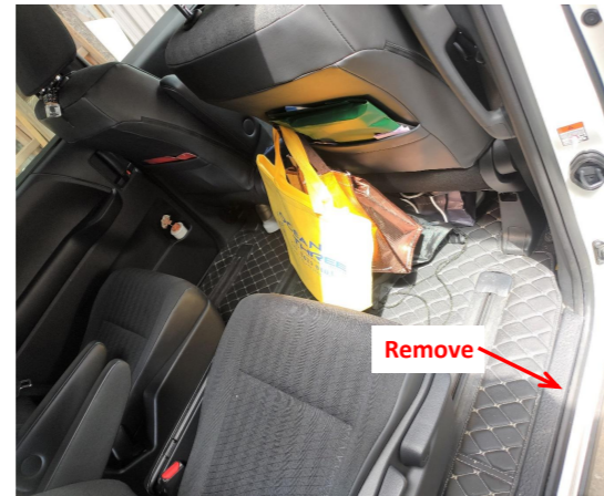
3. Remove the rear right door sill panel.
