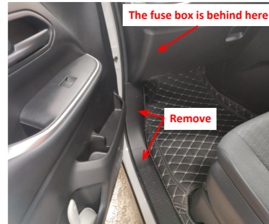
4. Remove the front left door sill panel and the trim panel on the right side of front passenger seat.
