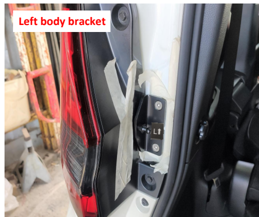
7. Replace the left body bracket.
