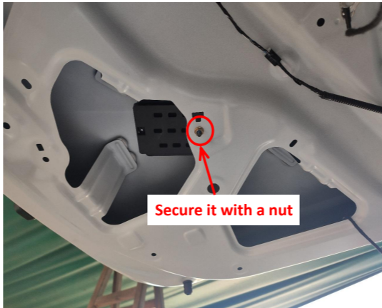
29. Place the ECU at the indicated position of tailgate and secure it with a nut.
