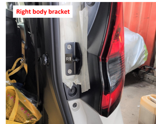
8. Replace the right body bracket.
