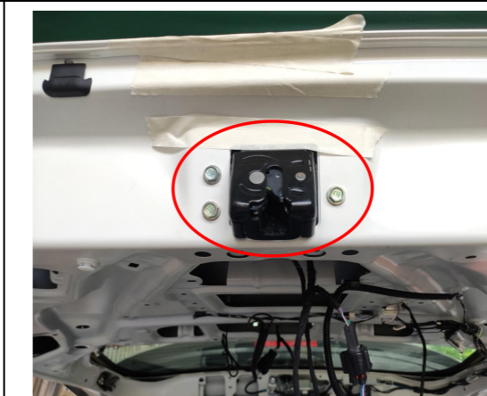
15. Remove the original latch and install the power latch.
