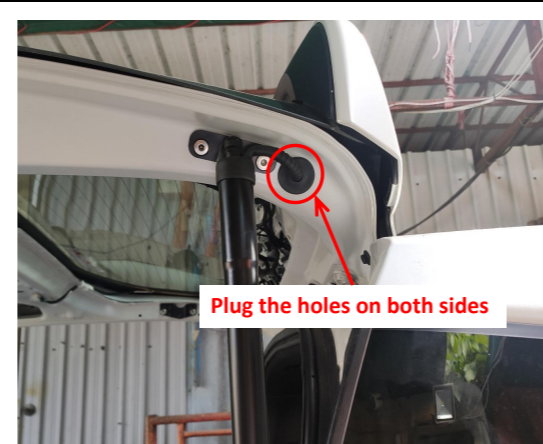
14. Plug the holes on both sides of the tailgate with hole plugs.
