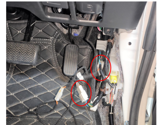
23. Connect the power harness to the signal plug and its socket beside the pedals.
