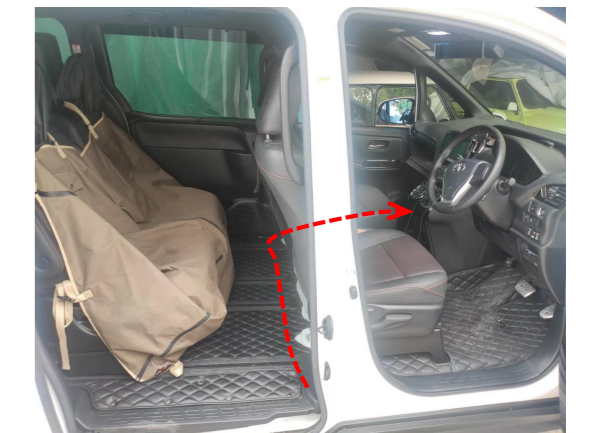
26. Route the fuse tap of the power harness from the rear seat to the front passenger seat.
