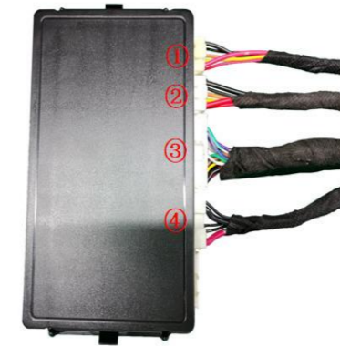
30. Insert the strut wiring harnesses ① ②, lock signal harness ③, and power harness ④ into the ECU in sequence.
