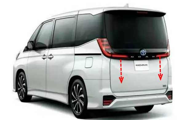
31. Press the added tailgate switch to open and close the tailgate once, the system completes initialization and then test each function of the electric tailgate.
