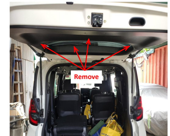
1. Remove the tailgate trim panels.
