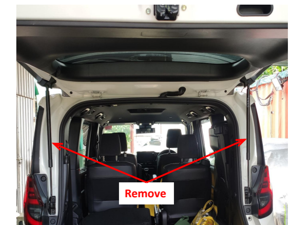
6. Remove the original gas struts.
