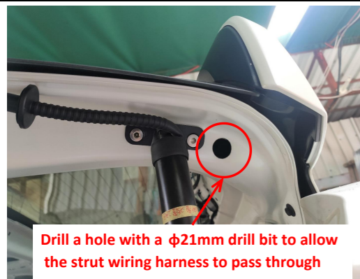
12. Drill a hole at the indicated position using a \phi 21\text{mm} drill bit to allow the strut wiring harness to pass through. Both sides are the same.
