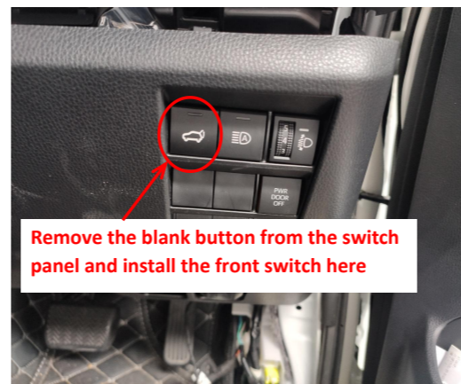
24. Remove the blank button from the switch panel and install the front tailgate switch.
