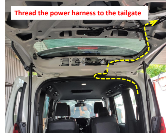
20. Thread the power harness to the tailgate.
