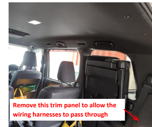
5. Remove the right side trim panel from the trunk to allow the wiring harnesses to pass through.
