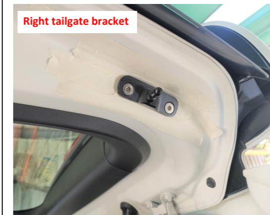
10. Install the bracket on the right side the of the tailgate.
