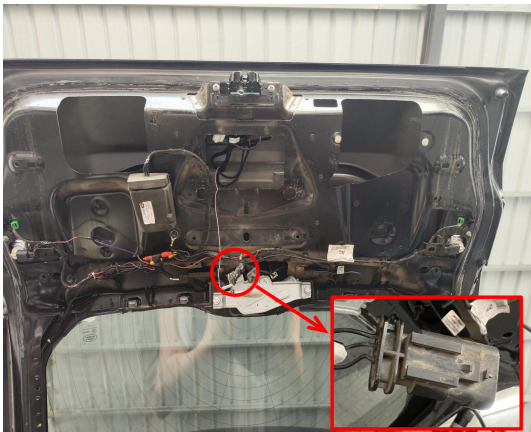
12. Connect the T-harness connectors of the lock signal harness to the connectors of the original tailgate switch.
