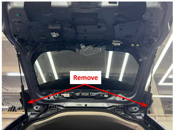
3. Remove the original gas struts.
