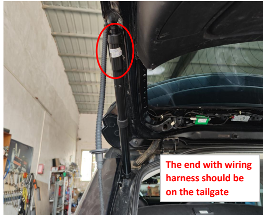
6. Install the electric struts, L on the left and R on the right (the first letter of the strut code).
