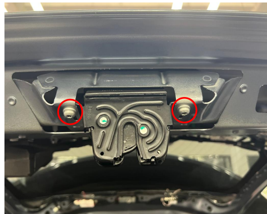
9. Remove the original latch.
