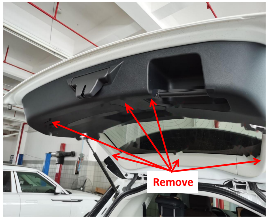
2. Remove the tailgate trim panels and screws.
