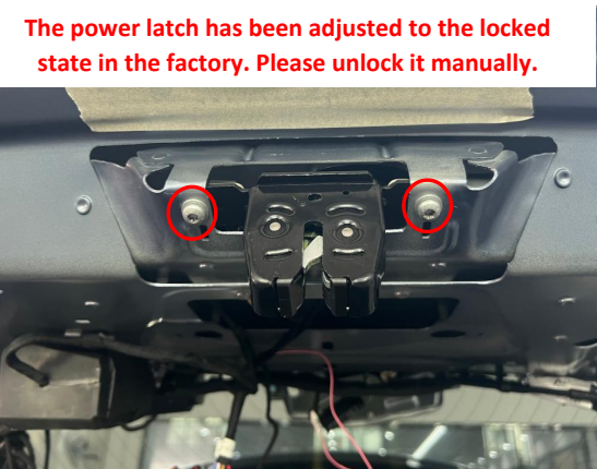
11. Install the power latch.
