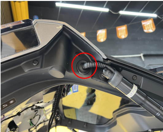
7. Remove the hole plug from the tailgate to allow the strut wiring harness to pass through.
