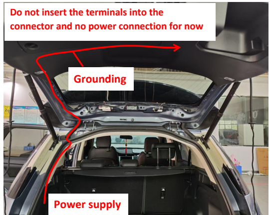
13. Route the power harness to the tailgate.
