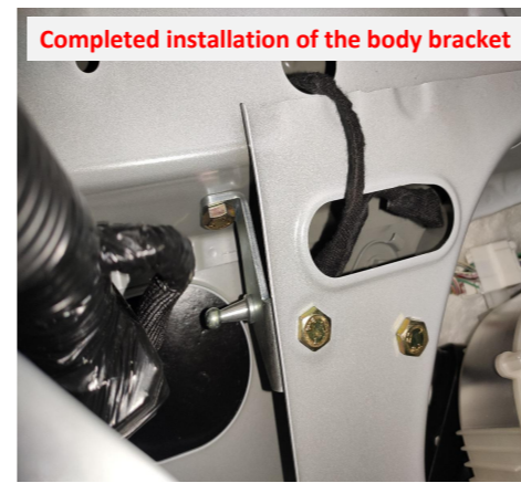
4. The completed installation of the body bracket. Both sides are the same.
