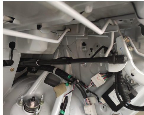
7. Install the electric struts, L on the left and R on the right (the first letter of the strut code), making sure the ends with wiring harnesses are on the car body.
