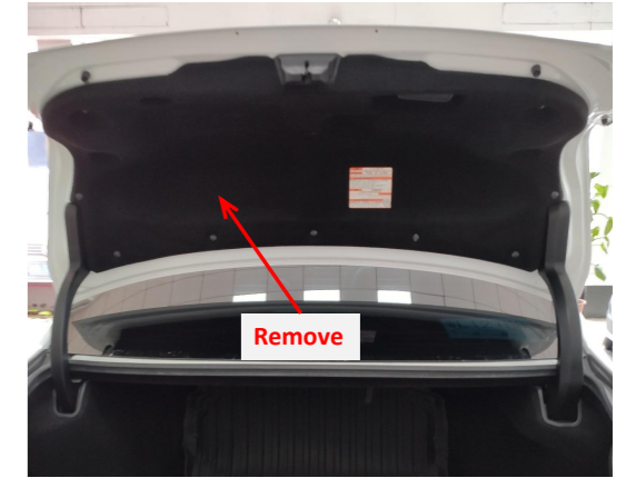
1. Remove the tailgate trim panel.
